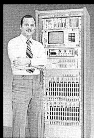
The Hawk Datatrap Model 4000 or 4010 lets you diagnose data communications problems quickly. Analyze protocol response between modems, terminals and computers. Visually monitor transmit and receive data and handshake signals. The Hawk operates on a wide variety of protocols.
