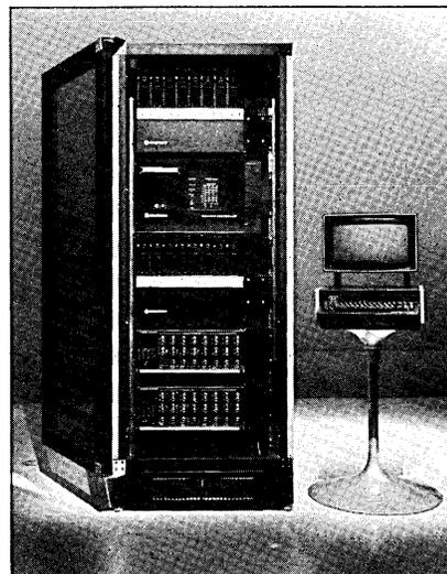
NETWORK CONTROLLER operates through a crt/keyboard terminal such as the Dataspeed 40/2 providing user of a large data communications system full diagnostic management of all Dataphone II service data in the network.
