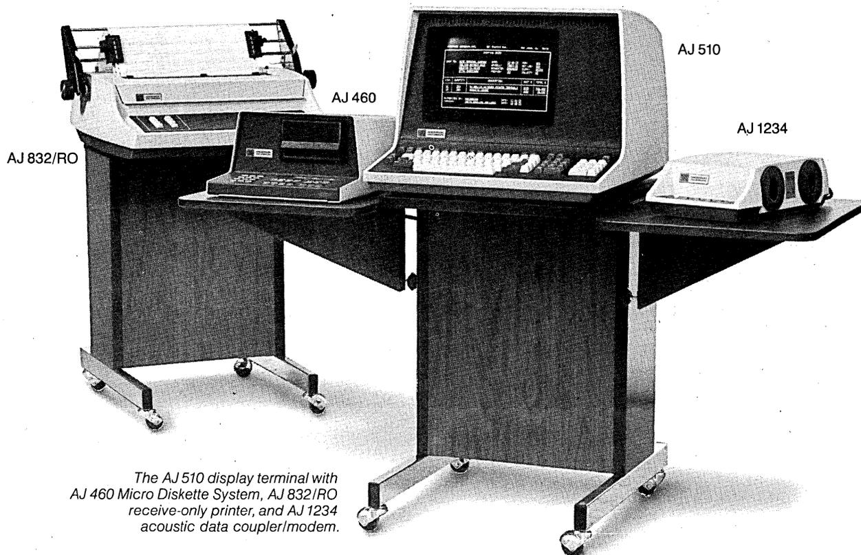
*The AJ 510 display terminal with AJ 460 Micro Diskette System, AJ 832/RO receive-only printer, and AJ 1234 acoustic data coupler/modem.*
