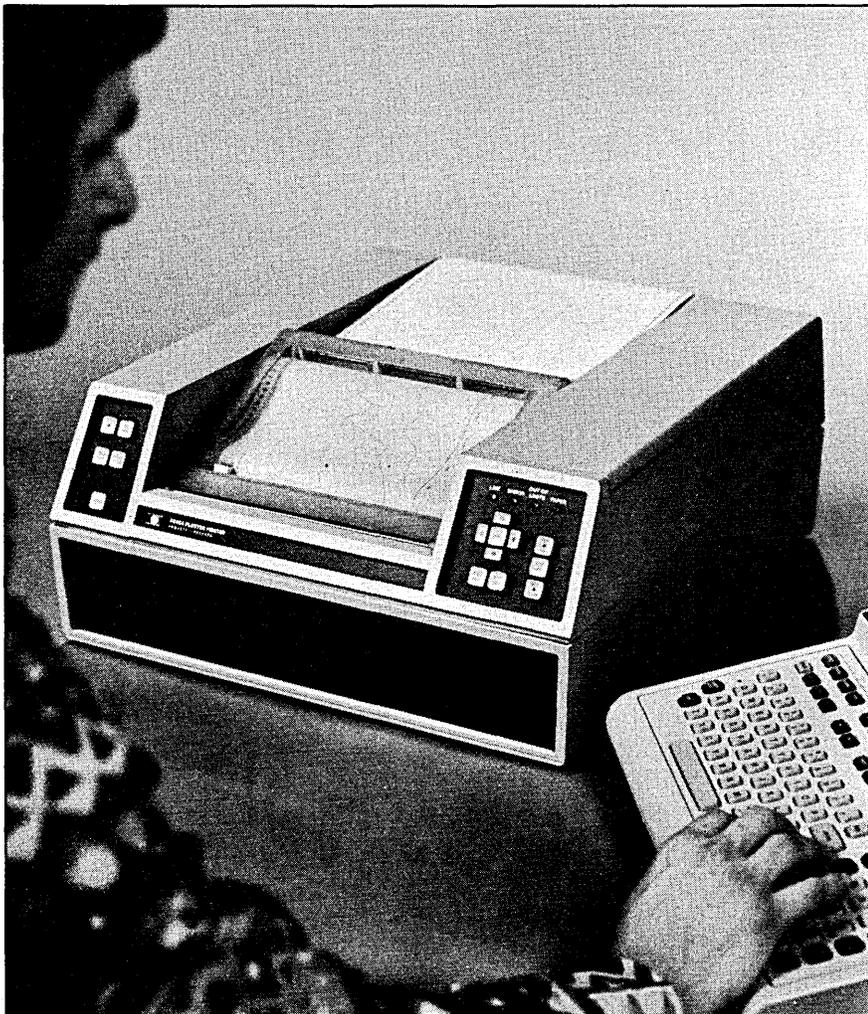
The basic intent of the crt dump printers is to provide a convenience copy of screen contents. To be effective in this role, they should be inexpensive, easily interfaced to their crt host, and quick. The thermal printing HP7245A is typical of the breed.
