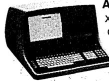
**ADDS Regent 200 Terminal** 24 lines x 80 characters, 25th "status" line shows operating mode. 128 character ASCII. RS232C/CCIT V.24 communications interface operating 75 to 19.2 BPS, switch selectable. Buffered transmission, auxiliary ports.
