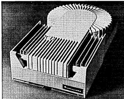
controller. The D160's sealed disk modules contain two platters for 60MB capacity, three platters for 90MB, or four platters for the maximum 120MB; the modules also contain four, six, or eight heads, respectively. Servo data, interlaced in each track, are used for head positioning. Oem pricing, for annual quantities of 100, runs \$3,085, \$3,355, and \$3,625 for 60MB, 90MB, and 120MB versions, respectively.
