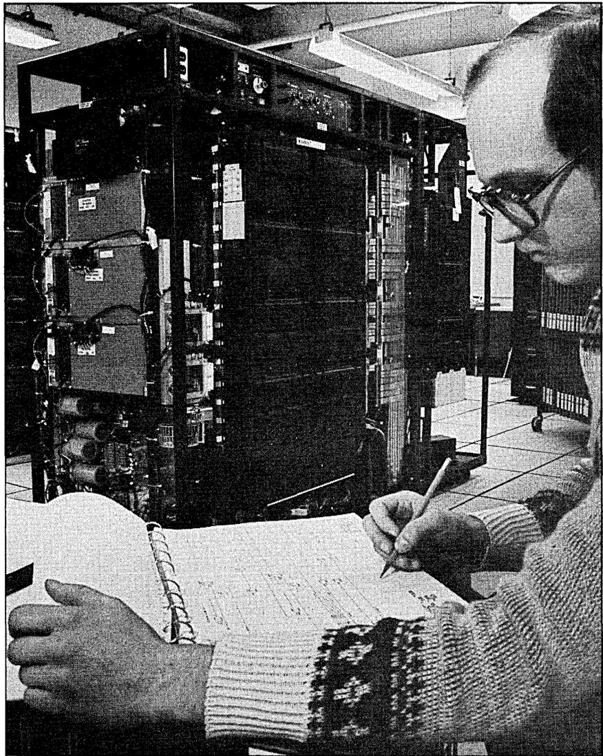
Good information on the channel directors is just now coming to the public, and this is one of the first photos to be released. Shown is frame five, which contains directors one and two (for the standard ration of channels). As can be seen, although the directors are logically "integrated" into the cpu, they are physically separate.
