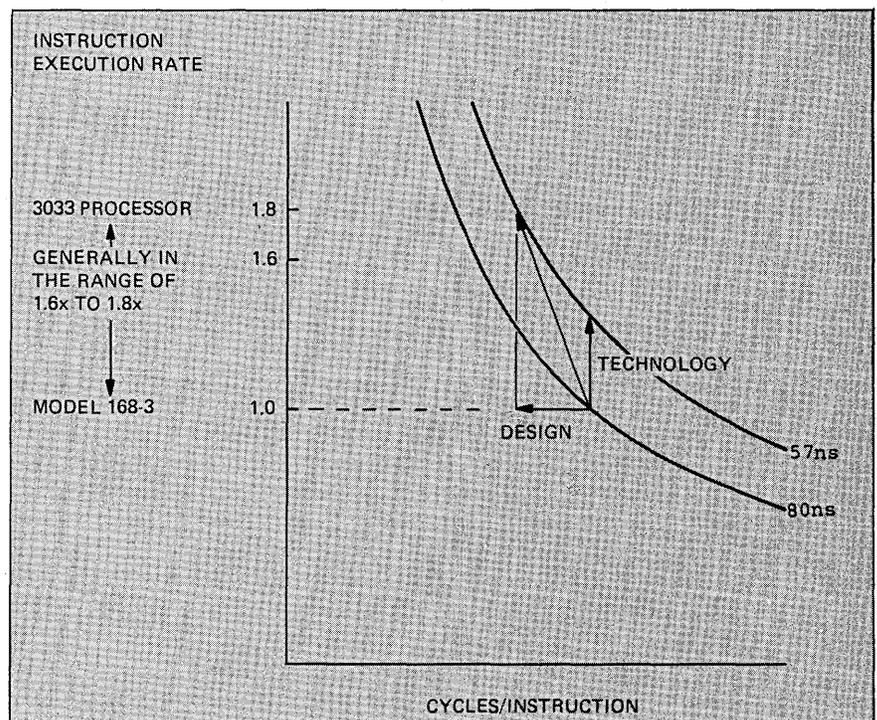
Fig. 1. A processor's internal performance is a function of technology and machine design. Thus the performance improvement of the 3033 over that of the 3168 is due partially to technology (reducing the cycle time from 80nsec to 57nsec leads to an increase in instruction execution rate of about 40%) and partially to design improvements which act to reduce the number of cycles per instruction.
