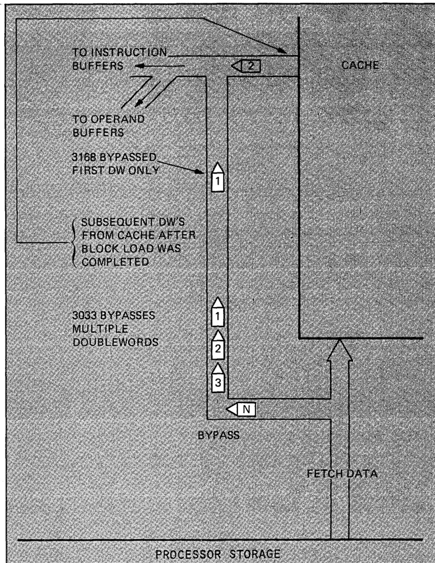
Fig. 4. When the 3168 required data which was not in cache, one doubleword was fetched directly from storage into the processor's buffers. The 3033 fetches several doublewords.
