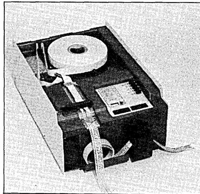
speeds are independent of each other. The dual-ported RS232 peripheral includes a 4KB buffer, automatic diagnostics, full- or half-duplex operation, and editing and duplication functions. Optional plug-in boards allow addition of more buffer memory or code conversion capabilities. The SRP-750 sells for \$2,695.
