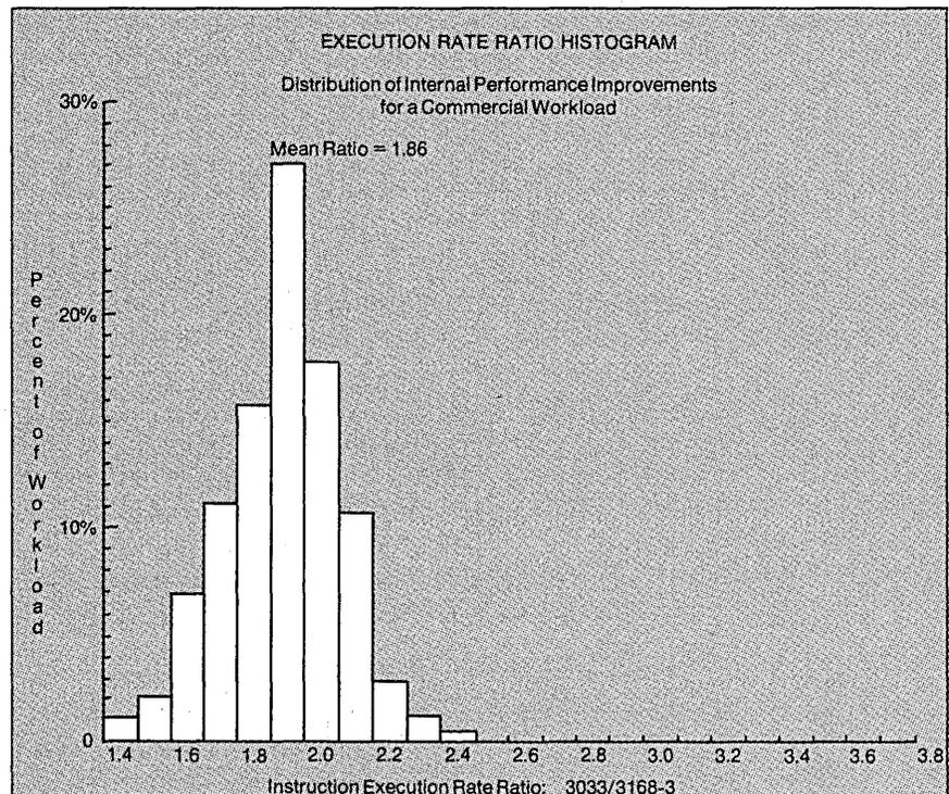
Fig. 8. According to a cycle by cycle simulation, the 3033 will run anywhere from 1.4 to 2.4 times as fast on a commercial workload as a 370/168-3 with the fast multiply feature.
