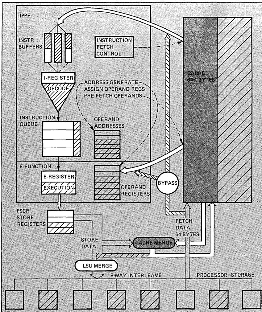
Fig. 2B. Changing the speed forces changes in the other elements as well, including adding to or lengthening buffers, registers, and cache for the 3033 (shown with crosshatching). Changes in instructions led to others in decoding and instruction execution as well.
