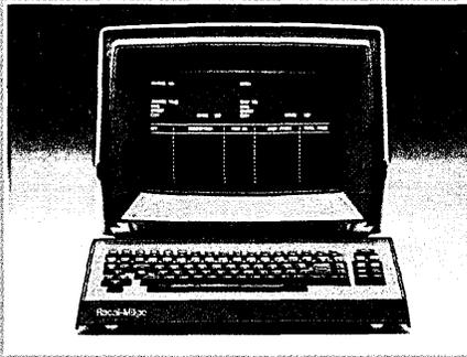
A full-featured CRT, plug-compatible with IBM 3275, to display and communicate your data at 4800 bps over dial-up lines and 9600 bps over dedicated lines.
