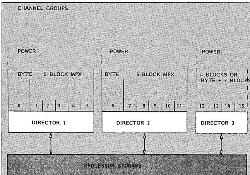
Fig. 6. Two groups of six channels each are standard on the 3033, and a third group of four channels may be added. Each group is controlled by a new element called a channel director, and, also unlike earlier processors, the channels are directly accessible by the service facility.
