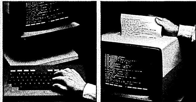
Try this on your favorite CRT! With the 2621P, you just hit a key and in seconds you have hard copy of your CRT display. The built-in thermal printer prints upper and lower case at up to 120 cps.
