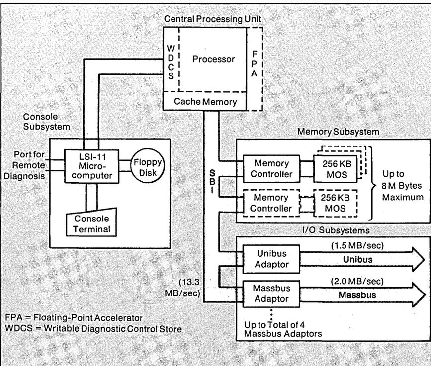
Fig. 4. The VAX design, as typified by its only family member thus far, the VAX-11/780, involves a microprogrammed processor, a built-in microcomputer, and a Synchronous Backplane Interconnect (SBI) for attaching memory and I/O devices. The architecture is based on a 32-bit longword; the SBI, the paths to memory and the I/O adaptors, and its 16 registers are all 32-bits wide. The 16-bit I/O channels streaming from the adaptors allow for the use of existing DEC peripherals.
