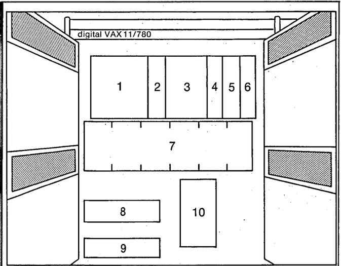
Components of this VAX-11/780 mainframe include: (1) the cpu, (2) Unibus adaptor, (3) 4MB of MOS memory, (4) and (5) Massbus adaptors, (6) slots for options, (7)
