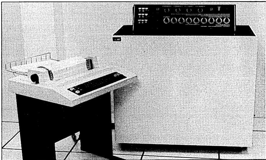
Cambridge Memory Inc. systems are available in two forms, a "full size" version of about 370/135 dimensions and this smaller one. The hardware which gets crammed inside is the same for either version: a processor up to 370/138 power, up to four channels, and up to 2 megabytes of memory. The system manufacturer is IPL, an affiliate of Cambridge, which also makes the Control Data Omega line.
