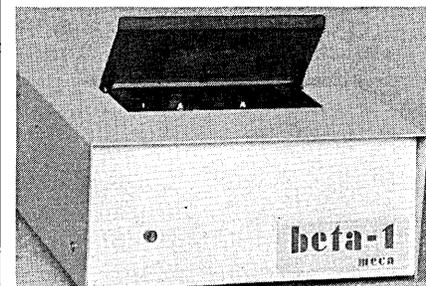
controlled unit avoids the constraints of any given bus structure by using an eight bit parallel interface; a serial interface can be had as an option. The Beta-1's data transfer rate is 8,000bps (16,000bps optional). The unit uses phase encoded recording, said to offer high reliability. An assembled and tested Beta-1 sells for \$399. MECA, Yucca Valley, Calif.
