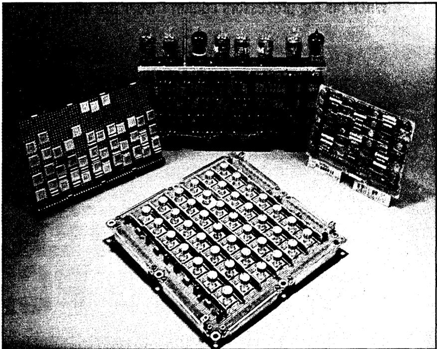
Dr. Amdahl has designed computers in all generations: first, vacuum tubes (IBM 704, background); second, transistors as discrete components (as in IBM 7030, board at right); third, integrated circuits (as in IBM 360, 370, and 303X, left); and current large scale integration (as in Amdahl 470, multichip carrier in foreground).
