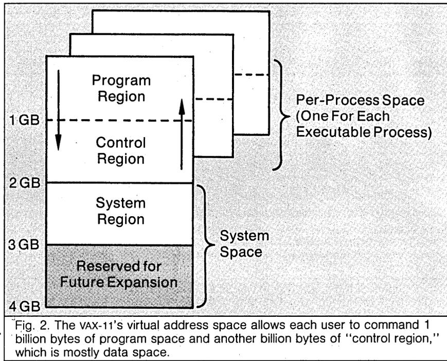
Fig. 2. The VAX-11's virtual address space allows each user to command 1 billion bytes of program space and another billion bytes of "control region," which is mostly data space.
