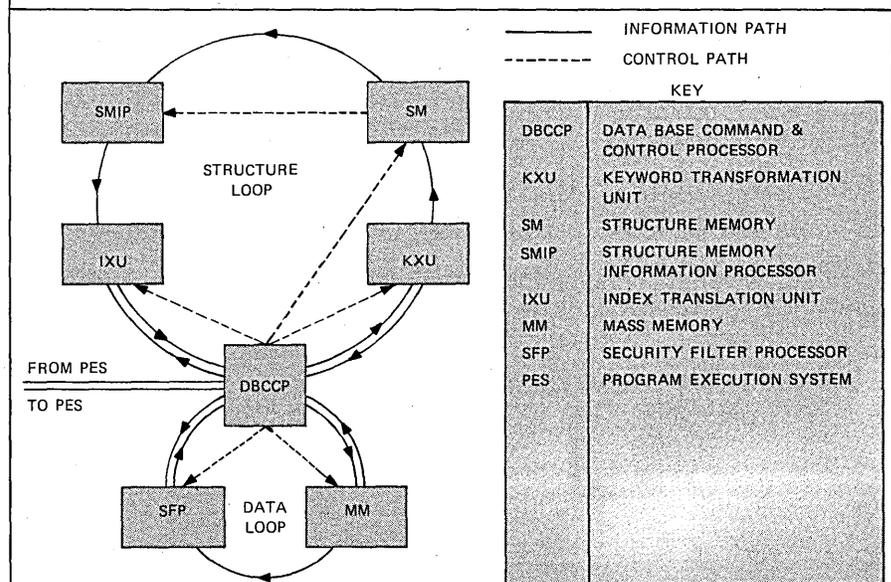
Fig. 4. The DBC (Data Base Computer) was designed to be a slave to a host cpu. It employs microprocessors for each disk track on a cylinder (one for each read head) so an entire memory may be read in parallel, and a pipeline processor architecture so that many processes may be performed on data simultaneously.
