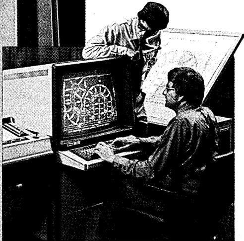
The 4016-1 can be optionally configured as a local digitizing station in conjunction with Tektronix graphic tablets and local storage devices. The user can digitize graphics data into a buffered tablet file with local editing capabilities. Plot courtesy of McDonnell-Douglas Automation Company. (Land system).
