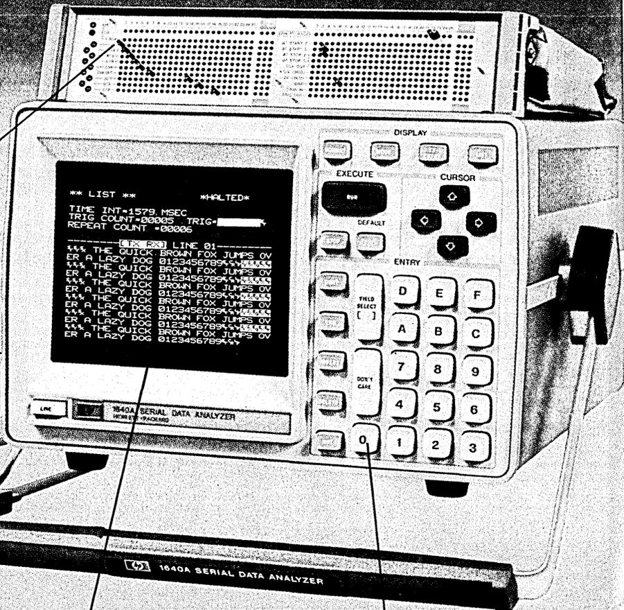
You don't have to be a programmer to use the 1640A; no instruction sets to learn... no writing or debugging programs. A menu set-up concept with keyboard parameter entry, pre-programmed measurement execution and transparent "wake-up" mode make the 1640A easy to use—even for semi-skilled operators.
