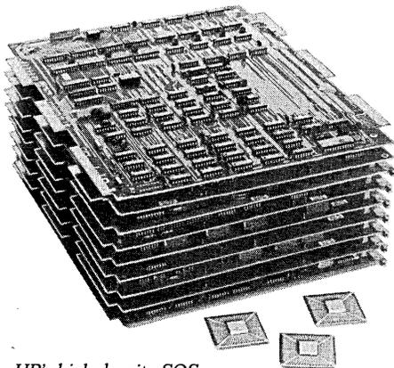
*HP's high density SOS technology reduced the 700 square inches of HP3000 components on portions of nine PC boards to three SOS chips. Results? Big computing power in a small package.*
