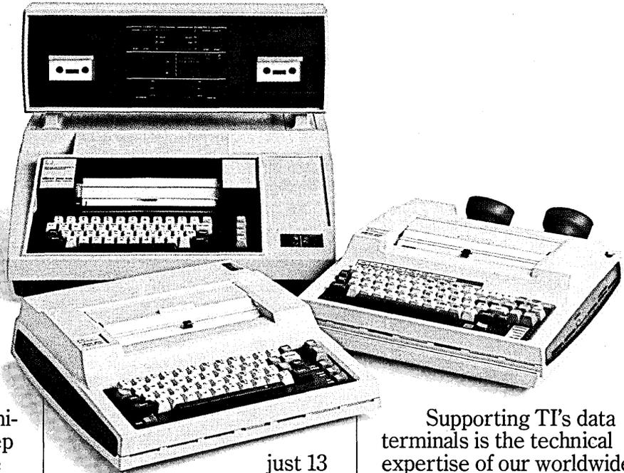
Our *Silent 700*\* Data Terminals really know how to keep quiet, even when they have a lot to say to your computer. All six models have virtually silent thermal printing, capable of printing up to 30 characters-per-second using their ASCII keyboards. And they all give you silent performance in different ways.
