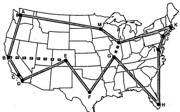
Tandem pass-through packet switching enables "A" to communicate with "E" at no penalty in system overhead. And you can add direct lines, per "B" to "E" or "L" to "G" whenever traffic warrants without disrupting system performance or efficiency. Note that nodes can be of variable sizes, all using Tandem NonStop Systems as the common element. Efficient, powerful and extremely low cost.
