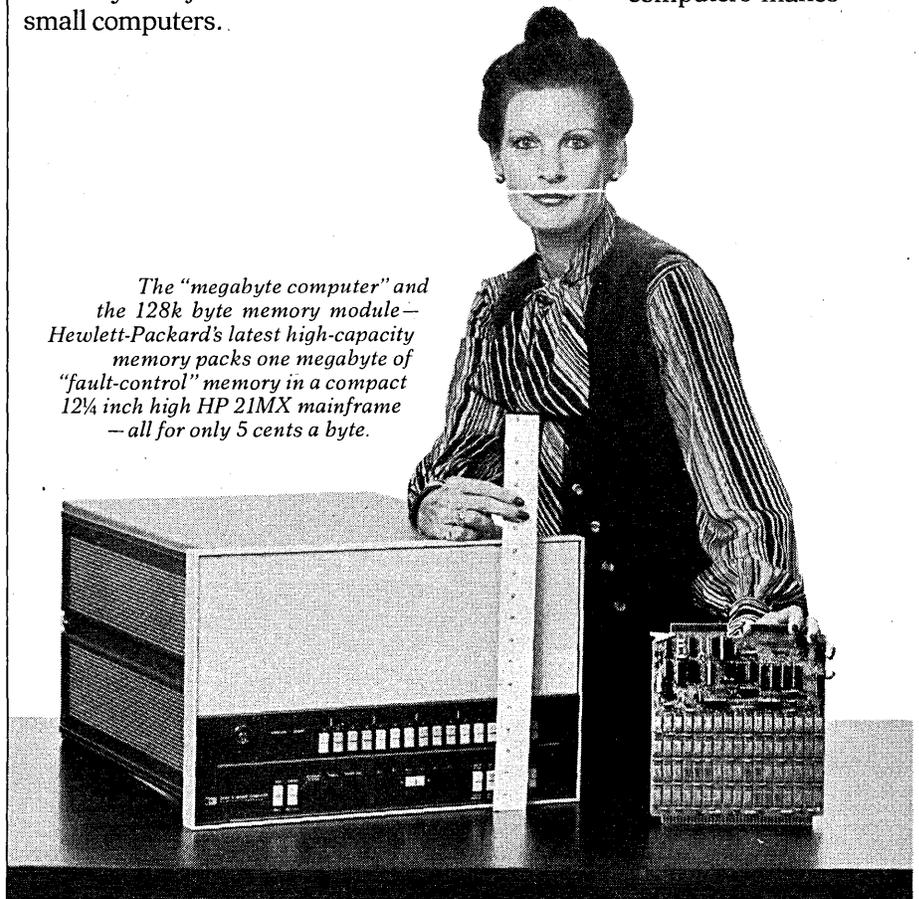
memory reliability a major contributor to overall system reliability. Recognizing this, Hewlett-Packard also introduced a new "fault control" capability, which provides for detection and correction of all single bit memory errors. This is accomplished through use of a standard 21-bit Hamming code. But, HP goes one bit further.
