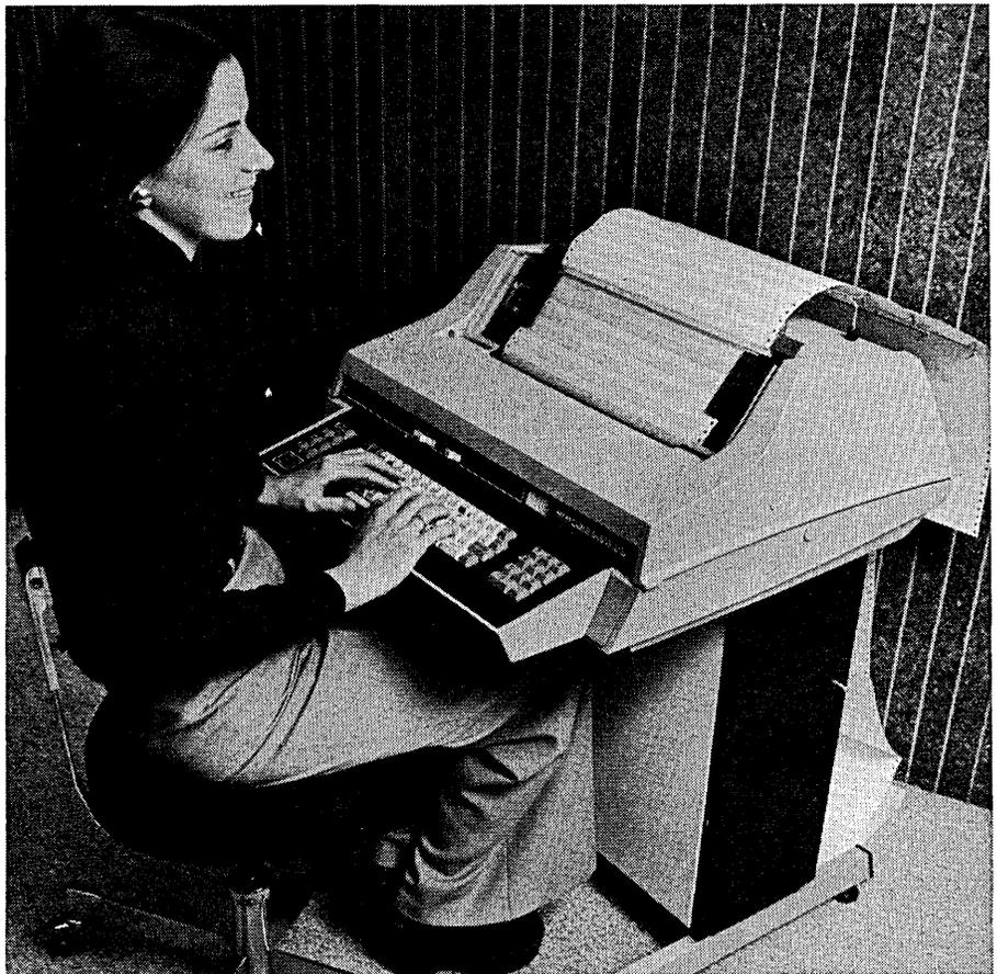
variety of configurations. It is available as a keyboard send/receive (KSR) teleprinter, shown above, as a KSR with magnetic tape cassette buffer or as a Receive-Only with our Video 100.
