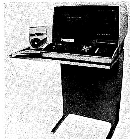
(on-line capacity 160KB). Synchronous and asynchronous communications are optional. A standard parallel printer interface allows connection of a hardcopy device, such as printers from Centronix and Diablo. Software includes an assembler, business BASIC, and a FORTRAN IV compiler. End user pricing for the basic Micral C is \$8,995; oem prices start at \$7,995. R2E OF AMERICA, Minneapolis, Minn. FOR DATA CIRCLE 306 ON READER CARD
