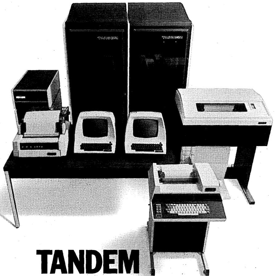
*The Tandem 16 NonStop System is composed of multiple, independent processors with dual redundant communications paths. The unique interaction between Tandem hardware and software assures not only continuous operation, and the integrity of your data base, but also throughput unmatched by any other computing system of comparable cost.*
