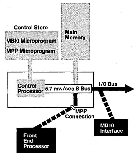
21MX E-Series provide for both I/O and processor growth power with two innovations: the Microprogrammable Block I/O (MBIO) and the Microprogrammable Processor Port (MPP).
