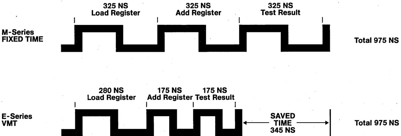
Thanks to a technique known as **VARIABLE MICROCYCLE TIMING** and other innovations the 21MX E-Series provides up to 100% performance improvement over the earlier 21XX family members. VMT dynamically defines the micro-instruction execution times. This results in time savings on shorter executing operations.
