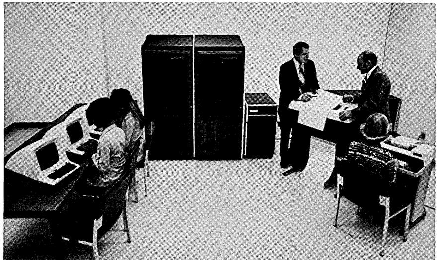
TANDEM COMPUTERS' NonStop computer system allows one processor to take over when another goes down. Now they're talking about an audible alarm.
