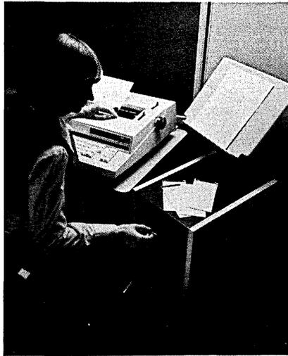
The Magna I electronic typewriter from A. B. Dick is typical of the hardcopy word processing systems now most prevalent. It uses a magnetic card for storage and a daisywheel print element, and is priced at just under \$10,000.
