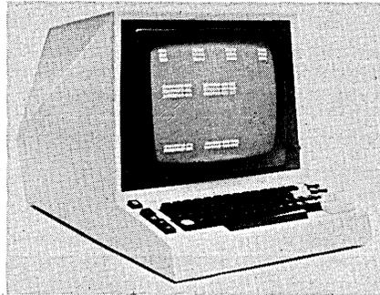
numeric pad, upper/lower case 96 character ASCII keyboard/display, switched serial interface for printer cassette or floppy disc, parallel input and output interfaces, and custom keyboard-character fonts for APL and French. Delivery is four to six weeks ARO, and unit prices start at \$1,595. VOLKER-CRAIG LTD., Waterloo, Ontario, Canada.
