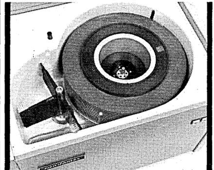
Alcohol and tongue depressors do not remove contaminants effectively. Usually they only spread them around and occasionally damage packs and destroy data as well.
