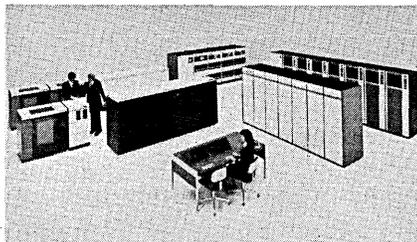
agement applications, multiprocessor performance/reliability," etc. Users can increase the processing power of their installations up to 50 times as they move from a B 6800 system to the largest B 7800 system, and performance is 2.5 times faster than the B 7700 system. The B 7800 clearly seems to be an IBM 168 or Amdahl 470 competitor.
