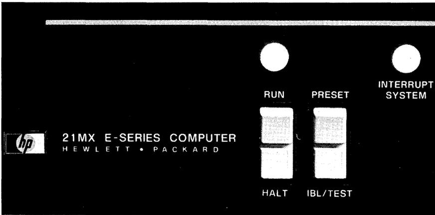
With the ease of a finger switch, a user can invoke a confidence check on 90% of the 21MX E-Series' circuitry.
