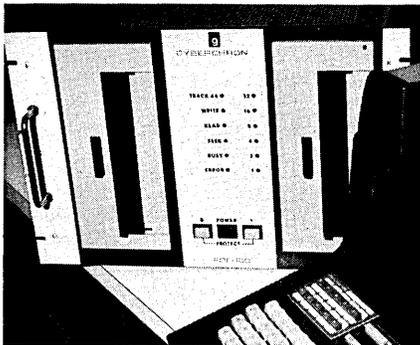
**MULTIPLE DRIVES** — Up to four disk drives on single select code — No additional select codes or cumbersome special characters required to perform drive selection. A simple software offset does the trick.
