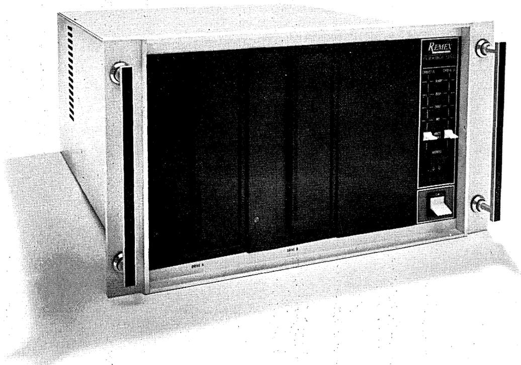
sector format.  saves computer time by data block transfer of from one to 65K 2-byte words on a single command from the host.  reduces core memory requirements due to automatic track and sector search and auto-initializing without software.  simplifies operation and system integration by 8-command structure.  saves space by housing interface card in the system chassis in some configurations.  speeds access through 6 ms track to track speed plus unit select.
