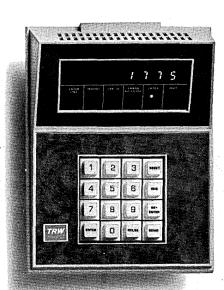
Entry and response. The simplest Digidata format—on the left—handles data entry, inquiry/response, and update of central files. Three response lights can be custom labelled for any application you need. In the more complex Digidata terminals, four or eight digits move from right to left, always displaying the last digits entered. They display numeric responses as well as status.
