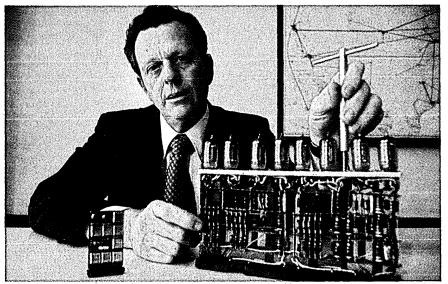
Bill Stringfellow explains how, through the use of a special tool, an eight-tube pluggable unit was set into a 701 computer. Alongside is an integrated circuit many times smaller, which performs comparable logic functions thousands of times faster in today's System/370.
