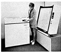
size of a flat-bed plotter. Like small drum plotters it moves the paper under the pen as well as the pen over the paper. Unlike small drum systems, however, it operates on paper up to 34½ inches wide, either in continuous rolls or in sheets (individual sheets get taped to a mylar sheet running between the two paper rollers).
