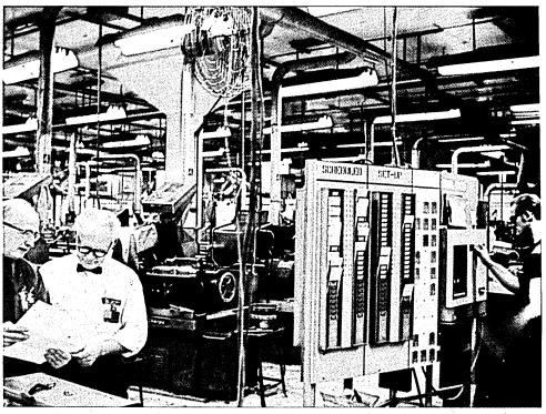
Punched cards follow the progress of each part being assembled in Allen-Bradley's Milwaukee plant. As each major step in assembly is completed, an employee inserts the part card and his badge into a data collection unit (right), and depresses a sequence of buttons to indicate the operation completed.
