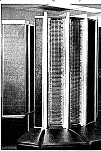
THE CRAY-1: Super computer designer Seymour Cray with Cray-1, a 64-bit machine that will sell for \$7.5 million with one million words of 50 nanosecond bipolar memory. Twelve columns hold 1,500 modules of memory and logic. Panels at right are removed to display how modules are arranged in two of the 12 columns.
