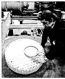
George Hefferon evaluates mirror optical quality. The honeycomb-like coring greatly reduces mirror weight by eliminating unnecessary glass.
