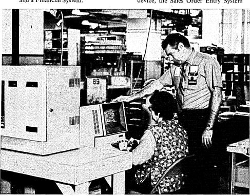
Variable length messages and inquiries are entered into the system at crt terminals such as this one in the stockroom. Such messages most often concern the flow of materials or orders rather than the status of a part being assembled.
