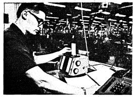
Auxiliary card readers, called "toasters" by their users, attach to the data collection terminals, extending access to the system while keeping the costs down.
