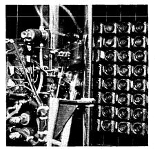
DOS/VS). It can be connected to up to four IBM 370 mainframes either with 3330 discs for staging data or through direct cpu connection.
