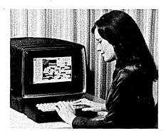
field blinking, and "blank video" to allow security codes to be entered but not displayed. Both 960 and 1920 character formats are offered, 12 or 24 lines of 80 characters.
