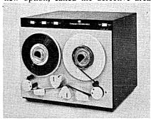
locator, allows the operator to more easily and precisely locate errors on tape. The unit operates at 180 ips. The price is \$2,200. COMPUTER-LINK CORP..
