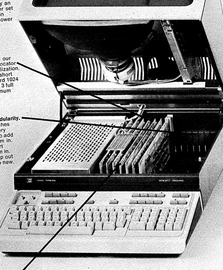
Computer-born microprocessor technology controls the show. An on-board microprocessor supervises memory allocation, data communication, keyboard scanning and display control.
