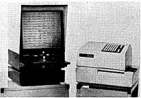
tion without manual coding or handwriting. The terminal, when connected to a punching unit, generates unique code numbers in man- and machinereadable form as items are selected from a microfiche menu displayed on the screen. Up to 5,400 printed item descriptions can be stored on one microfiche and presented as 45 pages of
