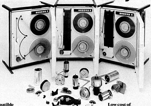
Compatible tension-arm and vacuum column tape drives.
