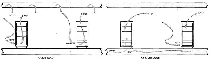
Fig. 3. How air is to be distributed is a separate problem. Overhead and underfloor plenums each have advantages. Underfloor ducting, for instance, is less susceptible to bad effects
