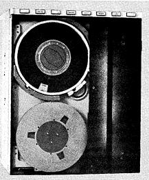
MOD 1200: Completely automatic tape loading with IBM wrap-around cartridge or standard open reel. Faster tape handling with longer tape life. Operates at 75 ips with all controllers using WANGCO's Mod 1100.
