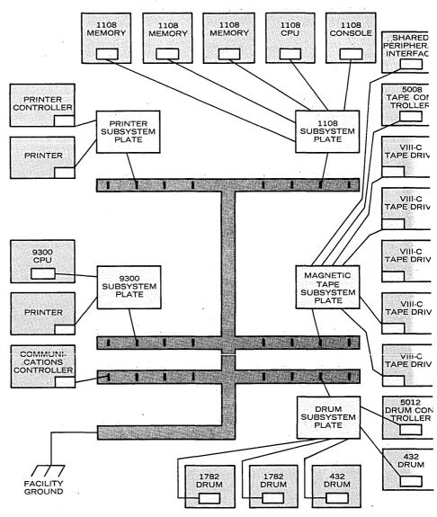
Fig. 4. Most electrical grounding systems have a single large central plate to which the subsystem plates attach. A central grid system like this one works better, but must be installed before other cabling, making it a poor choice for existing facilities.
