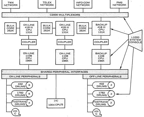
Fig. 1. InfoMaster centers are designed to accommodate over a half-million messages per day on TWX, Telex, telegram, and specialized business message service networks. The centers have three sets of Univac 418s and 1108s.
