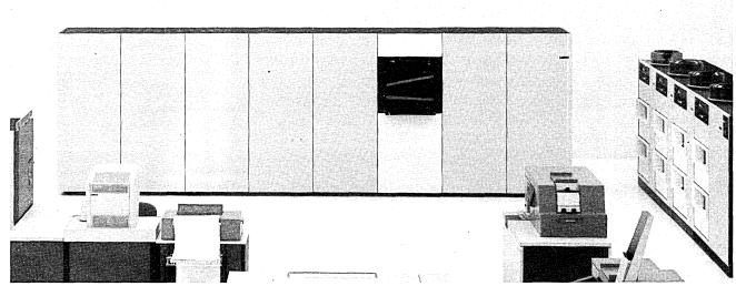
The IBM 3850 Mass Storage System, shown at the far end of this room, is linked to the IBM 3330 Disk Storage (right), which in turn is on line to a virtual storage IBM System/370. Maximum capacity of the 3850 system is 472 billion bytes.
