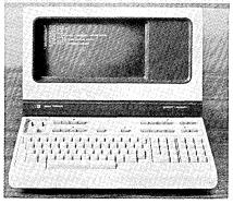
lines at a time by scrolling the 2640. Other features include self testing, plug-in character sets, dynamically allocated memory, inverse video, protected fields, etc. Having seen the terminal demonstrated, it doesn't seem like the vendor has left any conceivable option out of the 'order specification book. The interface is Rs-232c at switch selectable rates up to 2400 baud. First units go to the field during the first quarter of 1975. HEWLETT-PACKARD Co., Palo Alto, Calif.
