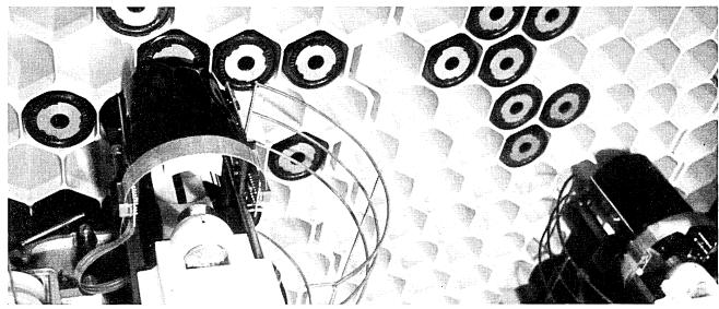
Inside the system, the cartridges are stored in a "honeycomb" of cells. When data is needed for processing, a cartridge is removed from its cell by an automatic mechanism and the data is temporarily read onto an IBM 3330 Disk Storage for computer use.
