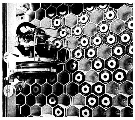
WHAT'S THIS? Inside the starship Enterprise's photon bomb magazine? No, this is a view of the IBM 3851 cartridge storage device. At left is one of two accessors in each system that move cartridges to read/write stations and return them to the "pigeon coop." A minimum 3850 system capable of storing 35 billion bytes rents for \$12,455, plus \$4,240 for the modified 3330 disc controller required.
