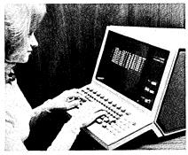
tape cassette unit, capable of storing 1.4 million characters is optional, as is a 30-cps hard copy output device. The Uniscope 200 sells for \$4,128 and rents for \$121/month. It is compatible with the earlier model 100 Uniscope. UNIVAC, Blue Bell, Pa.
