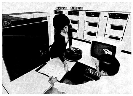
MODEL 158: IBM announced the 370/158 and other machines with virtual memory nearly 10 years after Burroughs offered concept with its B5000. But it wasn't until IBM began deliveries last year that the concept got wide exposure. Some see 158s and 168s accounting for more than half total dollar growth of entire 370 line.
