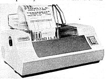
dling and warehouse system applications across many industries. Characters larger than the standard one-tenth inch are formed by assembling character sections or segments to make up any desired character under the control of a software routine. The 101S is priced at \$4,495 and is in production. CENTRONICS DATA COMPUTER CORP., Hudson, N.H.
