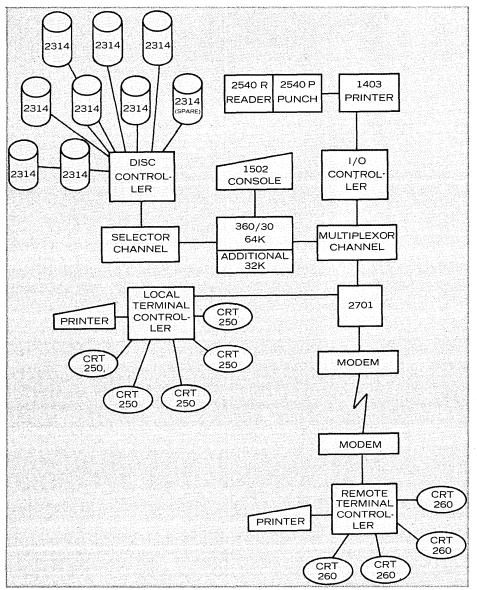
Fig. 2. After upgrading with additional peripheral equipment and memory, the refurbished "old" system operates at a fraction of the cost of a new one.
