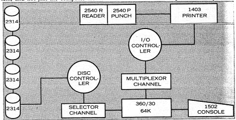
Fig. 1. The "before" situation in which the company's needs have outgrown the current system's capacity.
