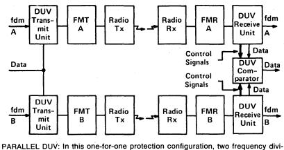
PARALLEL DUV: In this one-for-one protection configuration, two frequency division multiplexed signals and one 1.544 Mbps data signal are transmitted over two working radio channels. The comparator equipment then selects from the two decoded bit streams the one that has no bits in error.
