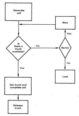
Fig. 2. A simple model of a telephone trunking system is adequate for investigating some call interarrival times, for predicting the number of lost calls, and for analyzing the effects of intermittent line outages.
