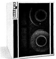
optional daisy-chaining. We've even succeeded in minimizing tape contamination by maintaining a positive pressure in the tape compartment area. And it's so quiet you won't believe it uses vacuum columns.
