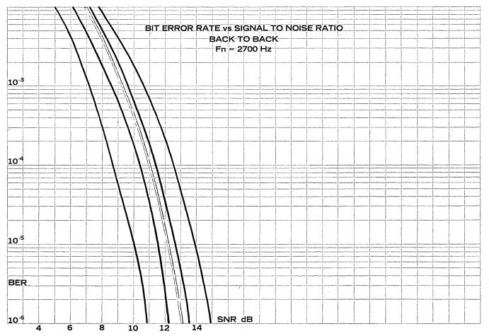
Fig. 3. The five brands of modems not eliminated by previous tests were then run in pairs, back-to-back. Although the curves look fairly close, the 201B modem, the middle line, is shown
