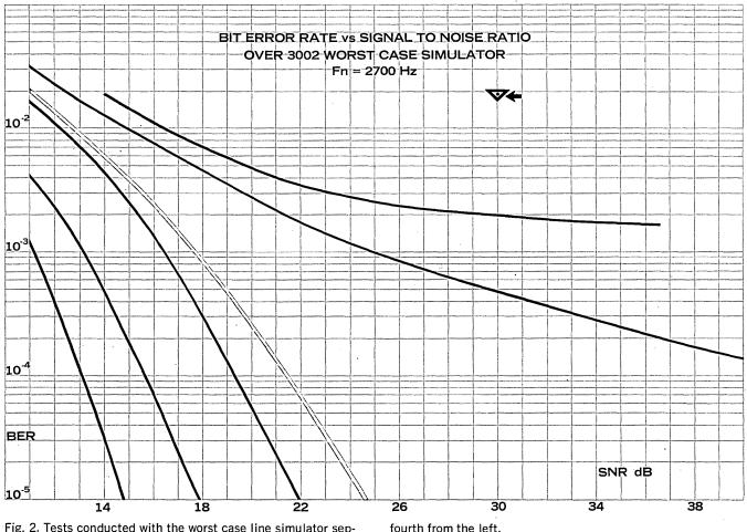
Fig. 2. Tests conducted with the worst case line simulator separated the modems by how well their line equalizers worked. The best curve is on the left. The Bell 201B equivalent is the
