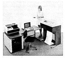
spooling, a standard on the system, makes it possible to input jobs from the 300 or 600 cpm card reader to disc, output another job from the disc to the 300 to 1800 lpm printer, and receive or transmit a third job over а
