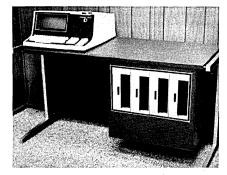
83 msec. The drive architecture features four 256-character buffers corresponding to sectors on the disc, giving a 1024-character addressable buffer, which should aid programming considerations. The diskette drive leases for \$110/month, with maintenance, on a two-year contract. FOR DATA CIRCLE 260 ON READER CARD
