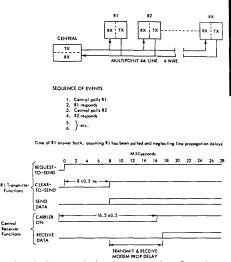
Fig. 4. Many of the Los Angeles County modems had to operate in a polled environment. This plot shows the timing sequence of a polled four-wire multipoint system. The remote site starts the sequence by raising Ready To Send signal. The central site master responds 8.5 msec later with a Clear To Send.
