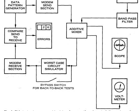
Fig. 1. This test setup was used to determine operating characteristics under various signal-to-noise conditions.
