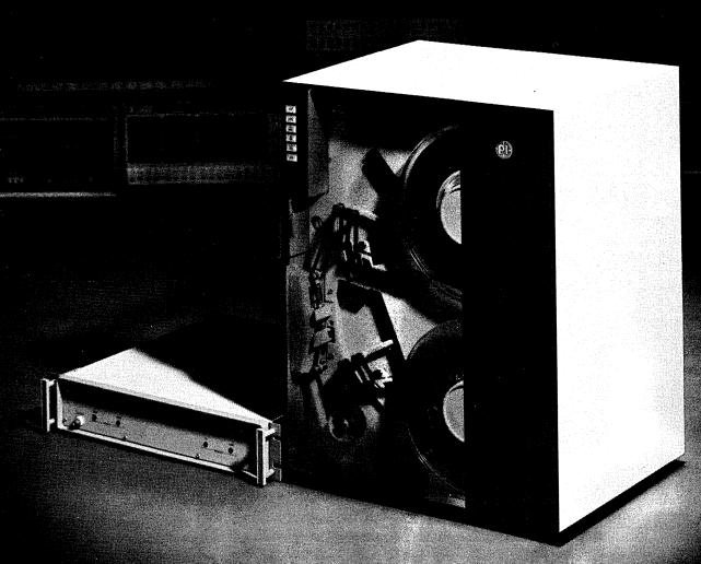
MINIMAX is our PI-1400, IBM compatible, digital recorder and hardware/software controller, matched to your minicomputer.
