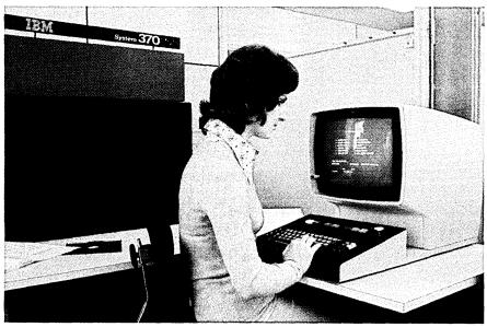
The Model 115 brings virtual storage to a new set of users. Also announced for all System/370s up through the Model 158 is the 3340 disk drive using the 3348 data module. This combines disk recording surfaces, access arms and read/write heads in a single cartridge, making for greater reliability and flexibility.
