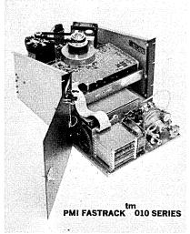
PMI produces a complete product line of high-technology head-per-track disc storage devices featuring high recording densities up to 6,000 bpi, that results in higher data throughput of from 4.5 to 51.2 MHz at a lower cost-per-bit for a given capacity-the 010 Mini Series with access times of either 8.5 ms or 17 ms and capacities from 1.2 Megabits to 19.2
