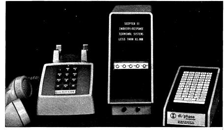
THREE-INCH CRT can display four 16-character lines and uses a 64-character keyboard.
