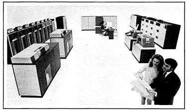
The new IBM System/370 Model 168 has a real storage capacity of up to four million bytes. It has the ability to handle 12 channels for high-speed devices.
