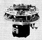
At the lower end of the storage scale, DATUM's Series 55 rotating drum memories provide 2K 16-bit word capacity with 18,000 bits per track on 2 tracks and an average access time of 8.3 milliseconds, for about \$650. Common capacities of 32K and 65K words run from \$1550 to \$1750 with self-clocked, read-write electronics.
