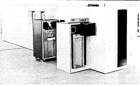
automatically scratched by generation or expiration date, and when the system calls for a scratch tape, the PDP-11 knows which one is the least recently used. And tapes are always transported to the nearest available drive. For tapes that are not cataloged, there is a pick-up port for these tapes to be entered when the JCL asks for the mount. In all, it seems to be a fairly well thought out product, requiring no changes to the host computer operating system.
