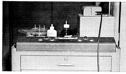
One component lives on. The high-speed paper tape reader has been modified to read into the 704 replacement for the ALWAC.
