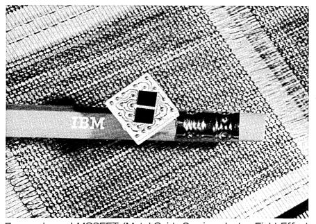
Four n-channel MOSFET (Metal-Oxide-Semiconductor Field Effect Transistor) chips the size of the two shown here provide the same 4K bits of storage as the core plane in the background. The chips run at twice the speed for half the price.
