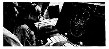
The STARAN<sup>™</sup> computer helps air traffic controllers achieve better management of controlled aircraft by automatically tracking *all* the aircraft in the sky. With STARAN, reliable ground-based conflict prediction and resolution is now practical and economical—no costly equipment is required in the aircraft. Truly, STARAN is a new computer tool—available now—to enhance air safety and to relieve costly congestion.
