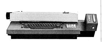
Tapes made on Novar off-line source data devices, including the 5-30 Automatic Tape Typewriter and 5-12 Recording Typewriter, can be transmitted via telephone lines by playing them on Novar 5-50 or 5-60 communication terminals. The 5-50 transmits in the Selectric correspondence code, the 5-60 in the ASCII code. Transmission rates available up to 2400 baud.
