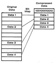
Fig. 2. Zero suppression by bit mapping.
