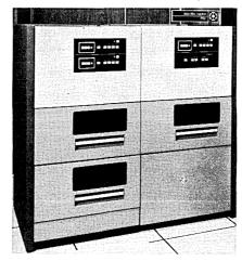
conditions as write error, head and/or cylinder error and its location, and drive not ready. A full 2314-equivalent (eight drives plus one spare, 233megabyte capacity) rents for \$3524 on a one-year lease, including maintenance and unlimited usage.-Delivery is 30-90 days. PERIPHERALS GENERAL, INC., Cherry Hill, N.J. For information:
