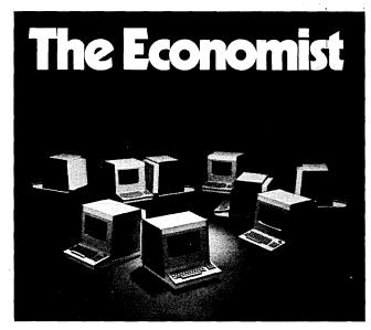
A 16 terminal Wyle 8000 CRT cluster costs between \$30,000 & \$40,000. An equivalent IBM 2260/2848 checks in at \$80,000 to \$100,000.
