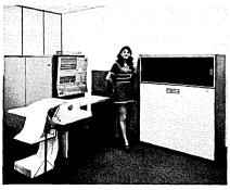
are 24X, 42X, and 48X for either 16mm or 105mm cameras. Push-button controls select the fiche format, which may be in COSATI, NMA, DOD, or custom formats. In addition to the standard 64-character EBCDIC 1403 array, a Katakana character set is available. Prices start at \$31,600 (\$888/month unlimited usage) for the on-line model, including prime-shift maintenance. Delivery is 90 days. CALIFORNIA COMPUTER PRODUCTS INC., Anaheim, Calif. For information:
