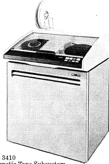
The 3410 Magnetic Tape Subsystem has been announced for most System/370s and System/360s as well as for System/3 Model 10, thus providing the Model 10 for the first time with the speed, versatility and storage capacity of tape.
