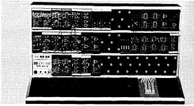
When Garrett Manufacturing Limited, Rexdale, Ontario, couldn't find a flexible, up-to-date lab trainer, the company decided to design one. The result was this MDL 1000 multi-purpose modular digital lab for demonstrating digital technology and bread-boarding complete digital systems. Teamed with Garrett's micro-computer, it is also an economical process control computer system.
