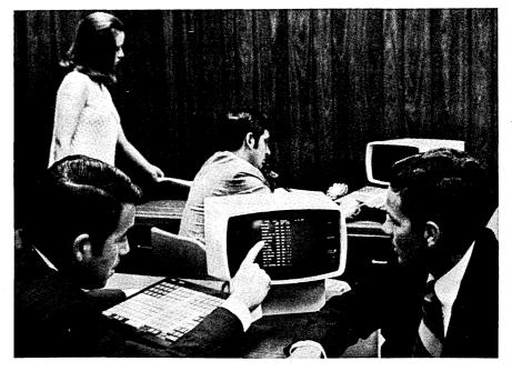
IBM's entry into the brokerage communications business gives a broker a grand total of 178 keys to push to call for data ranging from a customer's portfolio to current stock prices and to place orders that are automatically routed directly to the floor of the proper exchange.
