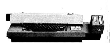
This is the new Novar 5-60 ASCII terminal that features a standard Selectric correspondence keyboard and type sphere, built-in 350 character buffer, built-in tape recorder, and a built-in modem. Transmission rates up to 2400 baud!
