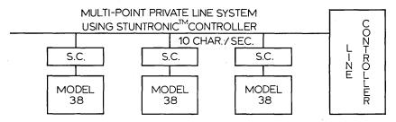
You can even use the model 38 in multi-point "selective calling" systems by adding a Teletype Stuntronic<sup>™</sup> station controller.
