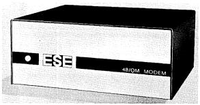
Latest innovation from ESE Limited, Rexdale, Ontario, is the 48/QM Modem which can signal at 98 per cent of the theoretical limit, ESE's experienced engineers have used specially designed filters which permit data transmission of 4800 bps in a channel bandwidth of only 1200 Hz over typical C2 conditioned lines without auxiliary equalization.
