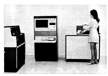
Configured as a communications terminal, the Mohawk Data SYSTEM 2400 can convert a tape that wasn't originally intended for communications, and then transmit it in a compressed, control-coded format.
