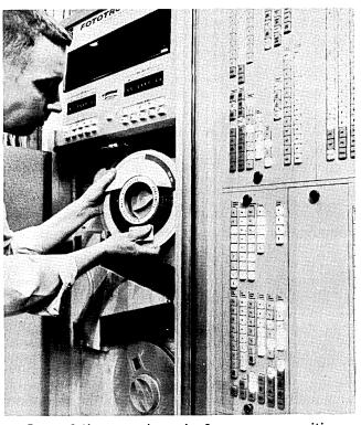
One of the new breed of area composition devices, the Intertype Fototronic-CRT is capable of outputting at thousands of characters a second fully formatted pages automatically with graphics in place.
