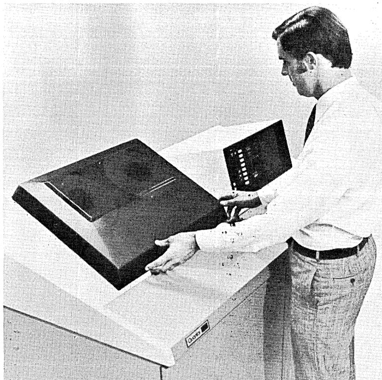
250 pages/minute, respectively. An installation that fills every page will slow the recorder down to 150 pages/minute. The 16mm film (up to 400 feet of it) is developed and delivered dry, packaged in a cartridge, and ready for use. Chemicals for the recorder come prepackaged in sealed containers.
