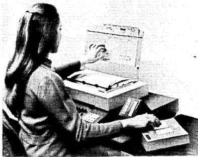
Ordinal numbers and additional keys for decimal point, plus sign, minus sign, asterisk, pound sign, field tab, and line return make up the 5-02 keyboard. The extra keys allow an operator to separate fields in a variable length record that might contain information such as payroll numbers, hours worked, hourly rate, and withholding information. The unit can be purchased for \$490 or rented for one year for \$15/month. For information:
