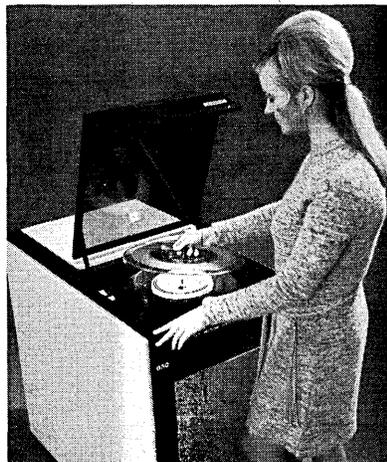
the DM-312 disc drive and the DC-314 which controls up to eight DM-312s on-line plus a spare off-line. Access times vary from 8 to 58 usec with 32 usec being the average. The same transfer rate (312KB) and capacities as the 2314 characterize the unit.
