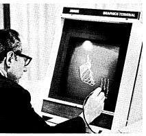
of programs. The user has access to the capabilities of the terminal via programs written on the computer. Image files are transmitted to the AGT for processing and display. Control files are used to activate the keyboard and the light pen, and to sample the function switches and any other interactive controls. The editor, assembler, and debugger are provided for support and maintenance of the communications and formatting routines.
