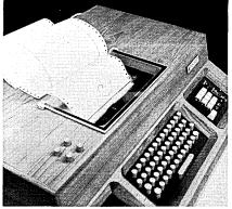
and knows some tricks that no one ever tried to teach a teleprinter. One of the most obvious differences-and actually one of the most minor-is that the standard tty keyboard has been augmented with a small numeric key set placed on the right side. The paper tape gear is, as expected, off to the left side.
