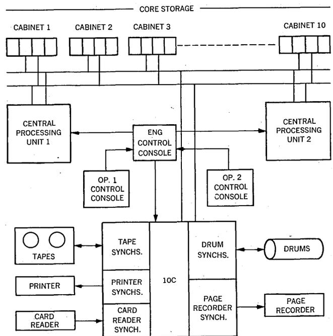
Fig. 1—Block Diagram of a LARC System
