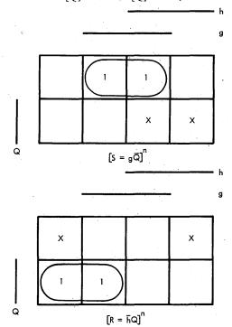
Fig. 6 Minimaps for the R-S flip-flop characteristic application equations.
