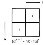
Fig. 3 Minimap for the T flip-flop characteristic equation.
