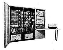
If you're looking for a computer system, SCC can give you 30-day delivery on a 660 CPU, a 1.75 usec memory with parity, memory adapter, character buffer I/O, 300 cps P.T. reader, 50 cps P.T. punch and Selectric typewriter with 8'' platen.
