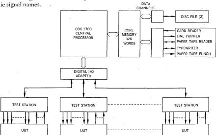
Production test system block diagram (above).
