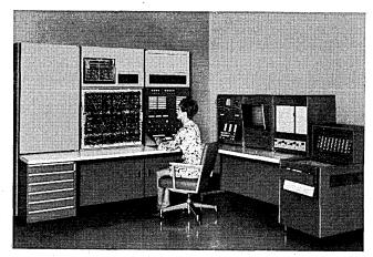
by adding plug-in modules. The console also has centralized master control and monitoring, central overload-indicator panel and automatic program hold. Computing components include a five-digit digital voltmeter, two-input electronic comparators, digitally controlled attenuators, gp registers and gp logic gates (AND, NAND, OR and NOR).
