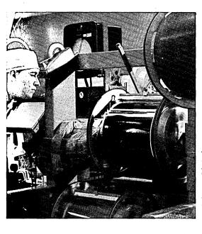
Ampex CATT computer tape is subjected to precisely controlled heat and pressure-ultra finished-to give it a non-abrasive, supersmooth surface.
