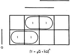
Fig. 8 Minimap for the T flip-flop characteristic application equation.
