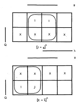
Fig. 9 Minimaps for the J-K flip-flop characteristic application equations.
