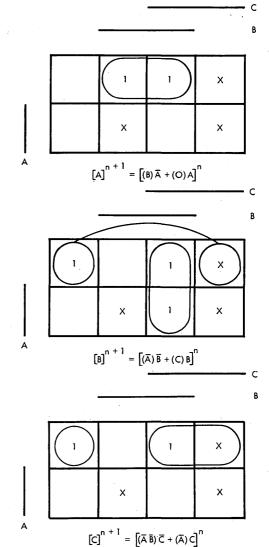
Fig. 11 Minimaps for the application of flip-flops A, B and
