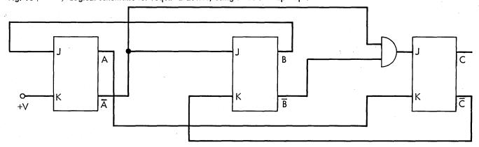
Fig. 14 (below). Logical schematic as in Fig. 13, but providing clock inputs.
