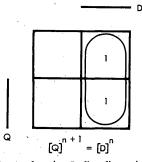
Fig. 5 Minimap for the D flip-flop characteristic equation.
