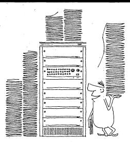
And that means more of it faster, and with less cost, work and worry. Raytheon Computer's \$15,000 703 has system characteristics built-in...1.75 usec cycle time...16-bit word ...memory expandable to 32K...byte and word manipulation ...real-time priority interrupt...options like direct memory access, multiply/divide, expandable I/0 bus.
