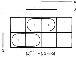
Fig. 4 Minimap for the J-K flip-flop characteristic equation.
