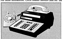
MATHATRON Much more than just a calculator, Mathatron has the capability to solve complex problems that are written directly with the keys. Mathatron can also be programmed and can make logical decisions.
