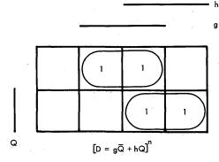
Fig. 10 Minimap for the D flip-flop characteristic application equation.
