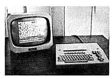
500 KC bit transfer rates is provided. The terminal, which operates in full-or half-duplex mode, is capable of incremental graphics and has Selectric hard copy as an option. For information:
