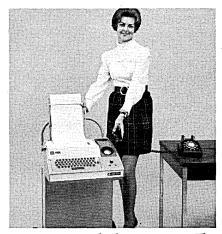
conversation with the computer. The ADT 233 is compatible with an ADC 300 terminals and 103A2 or 101C Data-Phones. The terminal is available with or without the paper tape punch and reader. For information:
