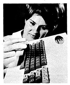
the encoding board has two vertical columns for each key while the reverse side has 32 horizontal rows of conductors. There are 16 possible combinations of a four-bit binary code (four zeroes through four ones). To form an eight-bit code two separate grid systems are utilized.
