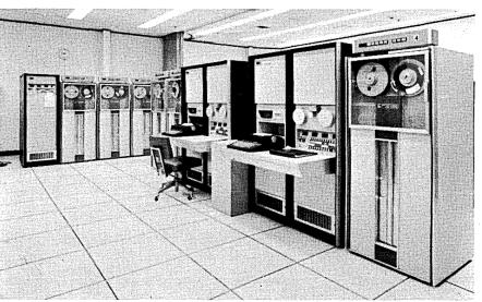
Raytheon 725Z computers, with Selectric typewriters, SC-1080 tape units, and Tally 424 paper tape readers.
