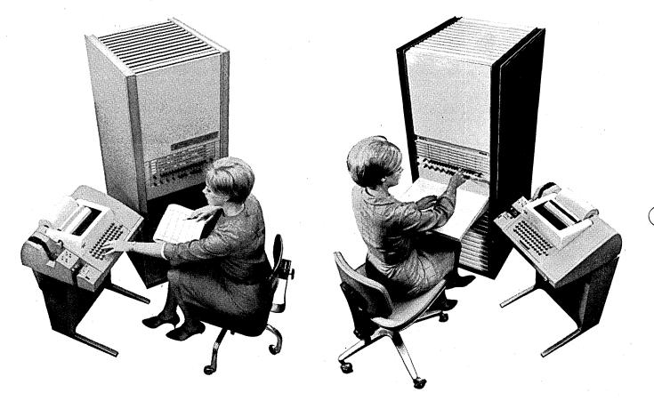
Over 50 SEL 810A, 16-bit computers have been supplied for data acquisition and control. Now meet the SEL 810B, with twice the speed of the A. Yet only about 20% more in price. Same great features: all integrated circuits, 2 levels of priority interrupt, memory expandable to 32K, I/O typewriter, high-speed hardware multiply and divide, and real-time I/O structure. And the software package of the 810B has been proven in the A.
