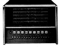
The 2115A has 16-bit words, 2  $\mu sec$  cycle time, 4K memory (expandable to 8K) and a \$16,500 price including Teleprinter.
