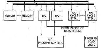
central processing units (CPU's) (1 to 3) to provide a multimission capability. The input/output (I/O) provisions are also modular to adapt the basic computer to a large variety of experiments and spacecraft. The memory modules are woven, plated wire, random accessed, and true non-destructive readout. Each module will provide 8,192 18-bit words of storage with a 2 microsecond cycle time.
