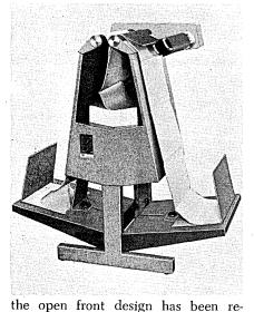
styled to permit design has been restyled to permit easier threading of form webs. Magnetic backstop plates allow location of form depths. Tines of carbon rewind forks have been connected into "U" sections to prevent operator injury. Speed of the decollator is variable, from 50-350 feet per minute, handling paper of 10-110 lb. substance. MOORE BUSI-NESS FORMS, Niagara Falls, New York. For information:
