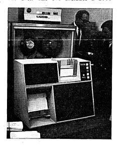
card hopper; the 310 has "recirculate" and "reject" off-set functions; 315 is the 310 with the 1,000 card hopper. The model 320 is the basic unit with a "step-column read" capability. Either 51- or 80-column cards can be read. Hopper capacity is 500 cards with a 1000-card modification available. Stacker hold 1,000 cards. OM-NITEC CORP., Phoenix, Ariz. For information:
