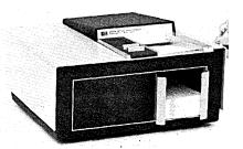
information. The unit, model 2760A, plugs into a standard telephone data set, and can be used in simple data communications applications. It operates in temperatures from 0° - 55°C and 95% humidity at 45°C. MTBF is 2000 hours at 25°C. A prototype of this model was displayed by the Datamec Corp. over a year ago, but did not perform to the company's satisfaction; now improved, it is being reintroduced.
