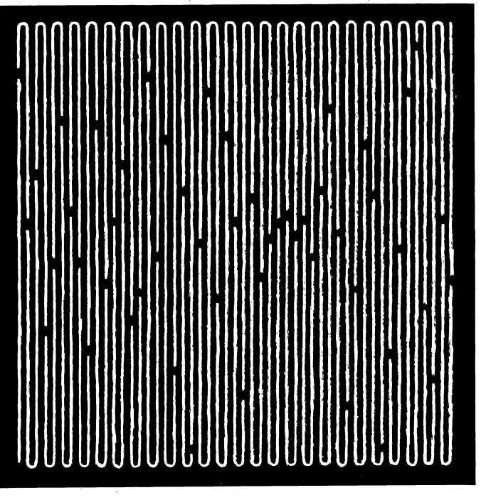
Just a few little bumps can make a magnetic tape a dropout.
