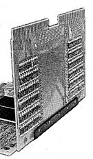
Scientific Data Systems – Sigma 2, 5 and 7 Computers 4K x 9 (opened); Sigma 2 900 nanoseconds; Sigma 5 and 7 850 nanoseconds; 23 mil cores;  $2\frac{1}{2}$ D.
