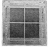
Northrop Nortronics—NDC 1000 Series Computer Development 16K x 14; 2 microseconds; 20 mil cores; 3 wire; 3 D.
