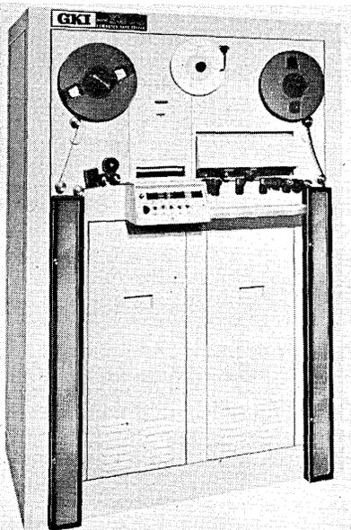
ment checks tape in a single pass operation, uses nine overlapping tracks in a 5 + 4 array, and has built-in cleaning devices. Modes of operation include evaluation, rehabilitation and certification.
