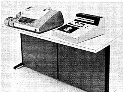
memory of 480 program steps. I/O devices include numeric keyboard, alphanumeric typewriter, punched paper tape, serial strip and page printers and electronic interface. MATHATRONICS DIV. OF BARRY WRIGHT CORP., Waltham, Mass. For information:
