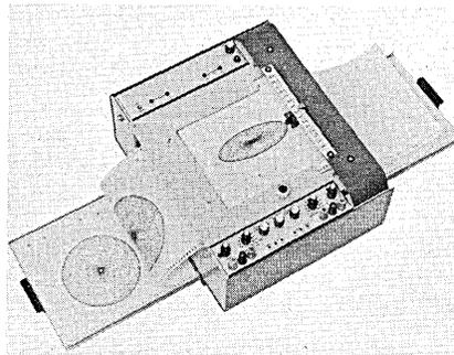
fan-fold paper, allowing a series of consecutive records without individual handloading of sheets. Mod 6650 is a bidirectional incremental plotter in which pen and paper move independently in discrete or incremental steps at speeds up to 18K increments per minute.
