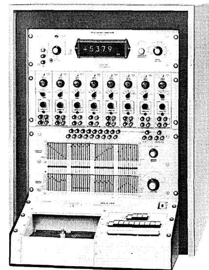
lyzer features crossbar switch programming, push-button test sequencing, built-in digital readout, universal test adapters, device protection, variable test time and modular construction. With an accuracy of 0.1%, the unit can test all standard i.c. packages.
