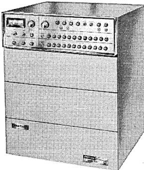
**CORE MEMORY SYSTEMS:** Speeds from 500 nanoseconds to 10 microseconds, 2½D and 3D organization. Use of integrated circuitry. Custom performance at "off-the-shelf" prices.
