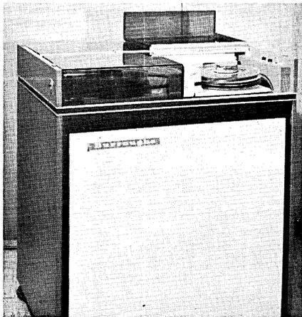
of pinch roller activity. Tape chamber is a sealed compartment; air flows through a micronic filter and is recycled 60 times per minute.
