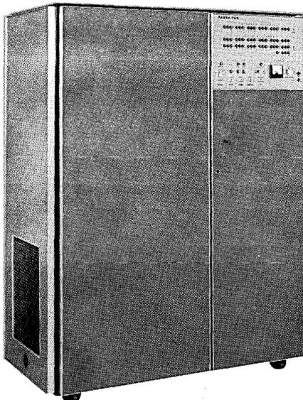
**MASS CORE MEMORY:** 2½D mass core storage at less than 2 cents per bit for 20,000,000 bits. Cycle times at computer speeds.
