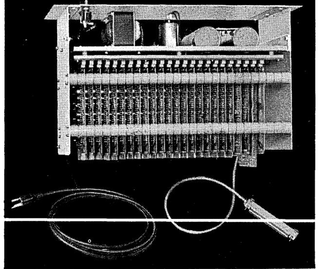
The Digitronics Model 5000 Block Reader Memory Module is all-solid state, compact, reliable and easily expandable. It can handle block lengths from 2 to 20 characters long with up to 8 bits per character.
