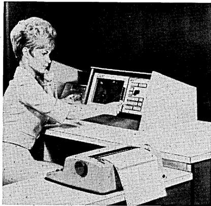
reader and paper tape reader. The recorder enables unattended transmission, which can be from a remote terminal to a computer center or to another terminal; the transmission is bidirectional. DARTEX INC., Santa Ana, Calif. For information:
