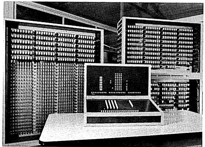
Z22's with electron tubes, and thirty-four transistorized Z23's.
