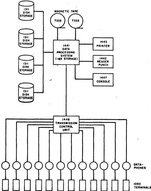
for this application. The IBM 1050 data communications terminal, shown in Fig. 2, serves as the input-output device for use by both authors and students. Presently, up to 24 students and/or authors can operate simultaneously on the same or on different courses. The limiting factor in adding more terminals to the system appears to be the amount of time delay that the student will tolerate between his response and the subsequent reply of the sys-
