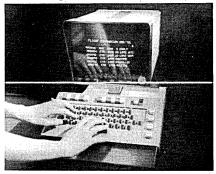
works with high concentrations of remote I/0 devices, and the 200's are general purpose units. The CRT's can display from 128-768 characters, and the codes conform with the ASCII standard. THE TELEREGISTER CORP., 445 Fairfield Ave., Stamford, Conn. For information:
