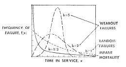
Varying one parameter (b) in the Weibull distribution function allows the characterization of many types of reliability phenomena.
