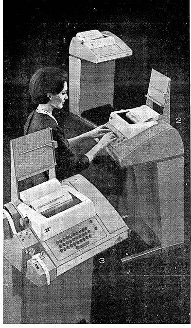
MODEL 32 SERIES. This new low-cost series operates at 100 wpm. Has a 3-row keyboard with a 5-level code. Shown above: (1) RO Receive-Only Set. (2) KSR Send-Receive Set. (3) ASR Automatic Send-Receive Set.
