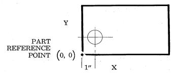
The planner must also specify once for the part, the relation of the part reference to the machine tool refer-
