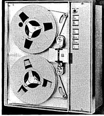
tape units, moving tape at a maximum rate of 100 0.005-inch increments per second. Rewind and fast forward speeds are 100 feet per sec. Price: \$5200. HONEYWELL, Denver Division, 4800 E. Dry Creek Road, Denver 10, Colo. For information: CIRCLE 207 ON READER CARD
