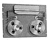
This is the new high performance Data-stor Model 110 perforated tape reader and spooler. Bi-directional tape speed: 400 char/sec. (other speeds available). Asynchronous stepping rates to 150 char/sec.
