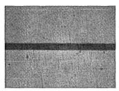
Accurately controlled gap lengths to 1 micron. Glass-filled gap permits mirror-like polishing, for smooth, optimum contact recording operations. (60x magnification)
