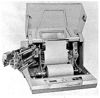
Destined for Lawrence Radiation Lab is the Radiation Series 690 "Super Speed" Alphanumeric Page Printer which achieves 31,250 120-character lines per minute, with a 64-character selection. (Datamation, June, 1963, p. 38.)
