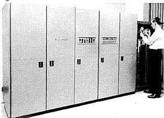
around 15,000 characters per second. The manufacturer states, however, that with only slight modifications it could handle speeds up to 90,000 characters per second. IBM's printer was built for the Social Security Administration to transfer tape files to microfilm. The system uses 16 mm film and handles input at speeds up to 6000 characters per second. Neither of these output devices produce hard copy directly.
