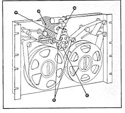
Mechanical simplicity... which yields a degree of reliability unattainable by any other paper tape reader! Simplicity made possible through the utilization of the revolutionary PMI printed motor direct drive servo. Movement of the tape through the read head is achieved by merely starting and stopping a printed motor. The brakes, clutches and pinch rollers that cause big trouble and down time in conventional tape transports are completely eliminated.
