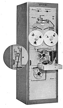
At 300 to 1000 characters per second of five to eight bits, the Tele-Dynamics system is the fastest paper tape presentation available for retrieving from and reading information into a digital computer or communications link. Printing electrostatically, it produces a permanent recording of coded information without mechanical punching, chemical processing, or paper burning. The reflected light reader reads both punched and electrostatic tape.
