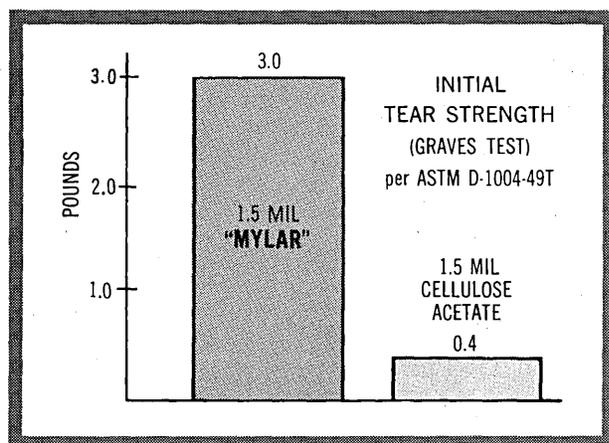
An unreliable tape can shrink or swell—cause garbled signals because the tape tracks shift laterally away from the recording and playback heads. With tapes of dimensionally stable "Mylar"\* polyester film you get accurate results . . . valuable programming time is saved.
