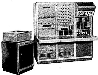
can test coincident-current memories of up to 16,384 words and word organized memory arrays holding up to 128 words, each with up to 128 bits per word. COMPUTER INSTRUMENTATION CORP., Route 38 and Longwood Ave., Cherry Hill, N.J. For information:
