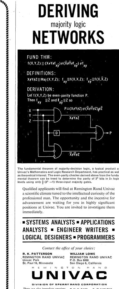
The fundamental theorem of majority-decision logic, a typical product of Univac's Mathematics and Logic Research Department, has practical as well as theoretical interest. The even-parity checker derived above from the fundamental theorem can be treed to determine the parity of 3<sup>n</sup> bits in 2n logic levels using only  $\frac{3}{2}$  (3<sup>n</sup> -1) three-input majority gates.
