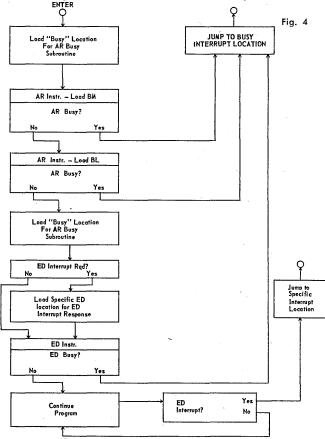
An external device interrupt will occur when an external device sends a signal to the central computer that it has completed its assignment. There are also provisions for two interrupt routines associated with a particular external device: one for normal interrupt and one for failure.
