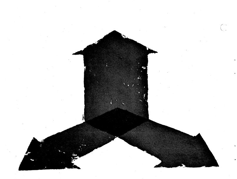
**Said Hans Oersted:** "When a conductor carries current through a magnetic field at right angles to it, the resultant reaction thrusts the conductor in a direction perpendicular to both the current and the magnetic field."
