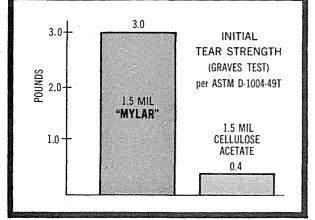
Every minute of downtime costs you dollars. That's why the reliability of your magnetic tape is so important. Tapes of Mylar\*, resist breaking from sudden starts and stops since they have high shock-tensile strength . . . and they have 7 times the initial tear strength of acetate tapes.
