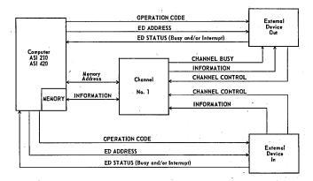
The EXTERNAL DEVICE CONTROL WORD (ED-CW) is present only during the ED instruction in the computer and when the address and operand are transmitted back to the device which if not "busy," sends a "start" signal to begin operation.
