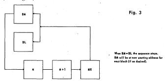
The Limit Address Register (BL) contains an address which is always one greater than that of the last memory location intended for a particular block data transfer by the respective I/O channel. BL may be loaded by the computer program through the use of the assembly register (B) instruction. BL cannot be stored.
