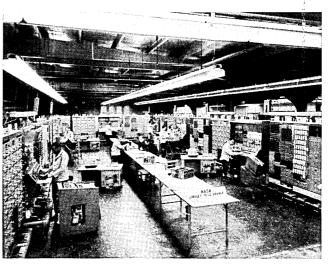
The world's largest general purpose analog computer, designed and built for the National Aeronautics and Space Administration, is seen undergoing final inspection and check-out at Electronics Associates, Inc. West Long Branch, N.J. All units of the computer were installed at NASA's Langley Field, Va., research center this spring. It occupies more than 1,800 sq. ft of foor space and comprises five separate PACE 231R computer consoles. CIRCLE 105 ON READER CARD
