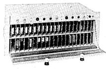
registers. Standard models are available with capacities of 24, 36, 72, 120, and 160 characters. Characters up to 6 bits in length are loaded serially up to 100,000 per second. Two manual operations are provided to facilitate maintenance and checking. DI/AN CONTROLS, INC., 40 Leon St., Boston 15, Mass. For information: CIRCLE 207 ON READER CARD
