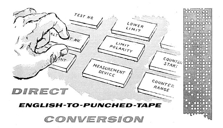
The McDonnell TAPE\* automatically prepares punched tape. TAPE's logic circuitry electronically analyzes word-group and numerical keyboard commands and converts them to complete coded programs. Punching mechanisms instantly deliver the finished tape. Editing, verifying, duplicating or correcting is accomplished quickly and automatically.
