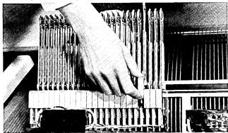
Access arms from IBM's new 1301 disk storage unit are easily removed for servicing.
