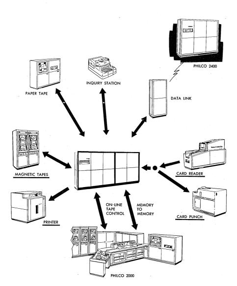
Expanded Philco 2400 for Data Traffic Control. Underlined captions comprise basic system: tapes, card reader, card punch, printer.
