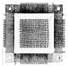
array. Compactness of design, achieved by wafer construction and by wiring memory cores on 50 mil centers, enables a reduction in stack dimensions. FERROXCUBE CORPORATION OF AMERICA, Saugerties, New York. For information:
