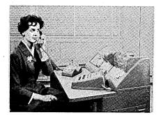
lar toll telephone calls – have been announced. The 7701 magnetic tape transmission terminal sends business and scientific data at the rate of 150 characters or thirty words a second. The data transceiver equipped with a dial-up telephone feature, can trans-
