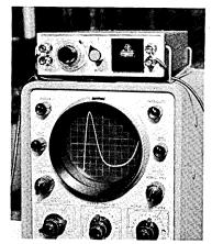
rather than just a portion of that curve. Through the use of an external decade box shunted across the horizontal terminals, it is practical to read the actual negative resistance of the tunnel diode at any point on the curve. For information write TEXAS INSTRUMENTS, 3609 Buffalo Speedway, Houston 6, Texas, or use card. Circle 216 on Reader Service Card.
