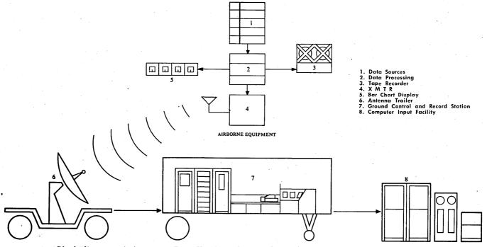
Block diagram of Automatic Data Handling System shows how airborne equipment, Ground Control and Record Station, and Computer Input Facility are integrated via telemetry link.
