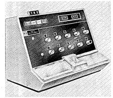
by computers to process such items as payroll, work-in-process inventory, costs and scheduling operations. The 180 Data Collector automatically assembles into a punched paper tape variable data (such as job-lot number and amount produced), identification data from pre-punched IBM cards (such as employee number & item number), fixed data (such as department number and Data Collector number), and time from an internal clock (to the nearest 0.01 hour). The
