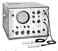
a single package, conceived to permit operation similar to a conventional oscilloscope. Model 185A has a rise time of less than 0.7 mus. Its full 10 centimeter vertical display and high
