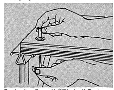
Exclusive Forsyth "Timlyn" Fastener produces a positive anchor of the floor panel to the V-LOK steel frame, yet permits removal of any section in minutes.
