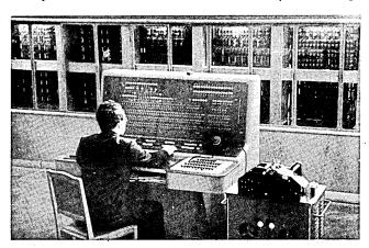
supplemented by 5,120 words on a drum. BESM II has more modern hardware and 2,000 words of core storage; the two machines are otherwise fully compatible. The core storage uses two cores per bit.
