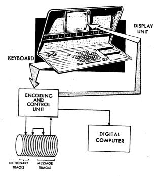
Figure 2. FLIDEN system block diagram.
