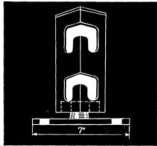
Quick Platform Leveling — the V-LOK column with adjustable base overcomes uneven floor conditions. Made in two heights — the  $11\frac{1}{2}$ " and  $7\frac{1}{2}$ " series.
