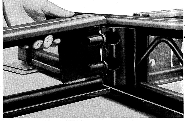
Engineered V-LOK Principle solidly locks the structural members of the computer platform installation into one rigid, quickly-assembled unit.
