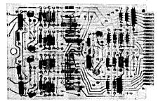
available from this manufacturer. FF3 contains 3 Eccles Jordan flip-flops. Non-linear feedback diodes are used to insure interchangeable operation without undue sacrifice of speed. Threshold bias provides noise discrimination. Clamping diodes are provided on both outputs to give a stable voltage level with low output impedence to minimize the effects of capacity loading. For information write DIGITRONICS CORP., Albertson Ave., Albertson, L. I., N. Y., or use reader card.
