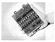
clad paper epoxy base laminated plastic. The plastic, EP-37, will not support combustion. A new adhesive secures the copper to the base laminate, so that EP-37 offers greater resistance to plating solutions. The new laminate will also withstand longer exposure to dip soldering at higher temperatures than XXXP-36. For information write FORMICA CORP., 4614 Spring Grove Ave., Cincinnati 32, Ohio., or use card.
