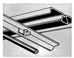
Instantaneous Wedge - Lock Bridging Fastener quickly secures purlins to girders without bolts or welds.
