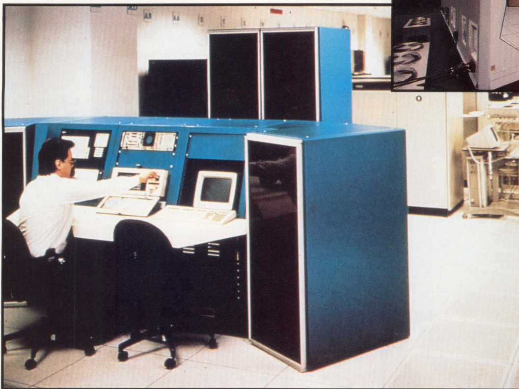
This mobile disaster recovery center, above, provides a 2,000-square-foot computer-ready environment, including a raised floor and a fire-protection system. Hot sites, such as that pictured at left, are complete data centers ready to take over your operation in the event of a computer disaster. Here, a clustered 8700/8810 resides behind a network control center that can handle communication needs.
