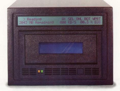
et the tape backup system that makes it easy to find out the facts. Our CY-8200 has a 2-line, 40 column LCD option that gives you *complete* status information. In easy-to-read, precise format, you see transfer rate, command under execution, unused tape in megabytes, and the ECC rate indicating backup integrity. No guesswork... just the facts.
