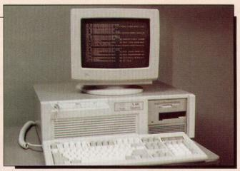
Soft-Switch's X.400 Gateway is a 386-based unit with network adapters for X.25 and SNA networks.
