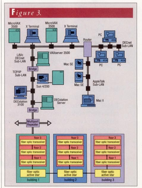
Fiber optic backbone supporting extended LAN.
