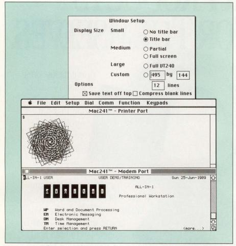
Figure 1: New features in Mac241 include multiple concurrent sessions, resizable and movable display windows and an optional vertical "save-text-off-top" scrolling bar.
