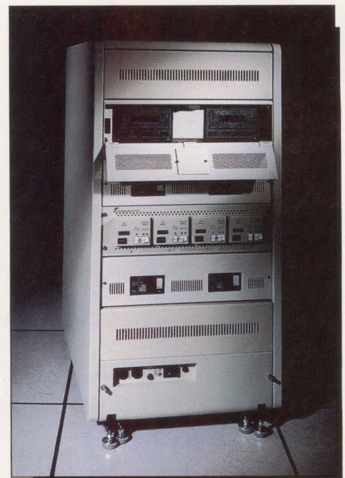
The SI2046 power pack holds up to four 8mm drives, each with a capacity of 2.3 GB.
