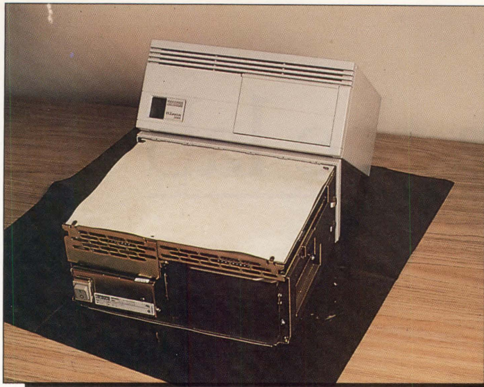
1: Top cover off — CPU is in the top layer. Don't forget static protection.
