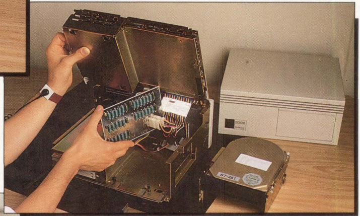
2: There is a resistive load card to remove. This uses up the power if there are no drives present. It's not necessary to remove the card, just unplug one of the power cables for your new drive.
