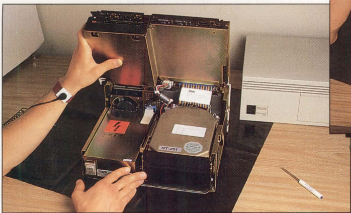
5: Time to button up. You format the disk by typing T70 to the >>> prompt. You can use T71 as a non-destructive verify after formatting.
