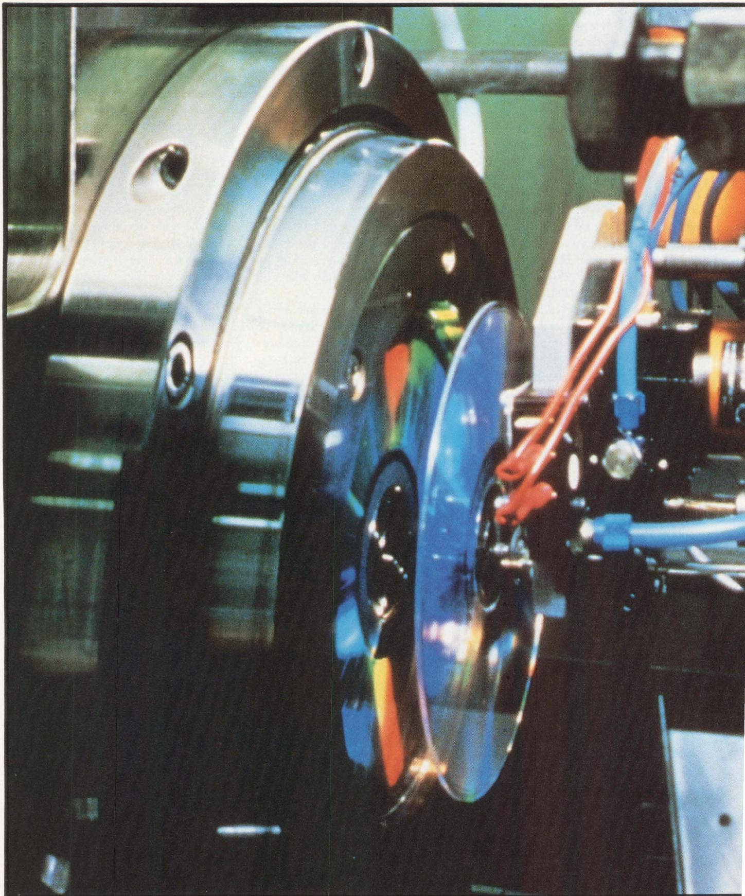
Injection molding process during the manufacturing of Plasmon Data Systems' WORM disks.
