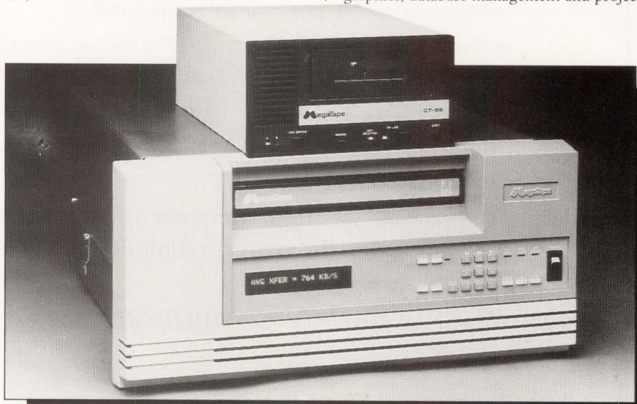
The GT-88, from MegaTape Corporation, is a high-capacity drive using an 8mm cartridge.
