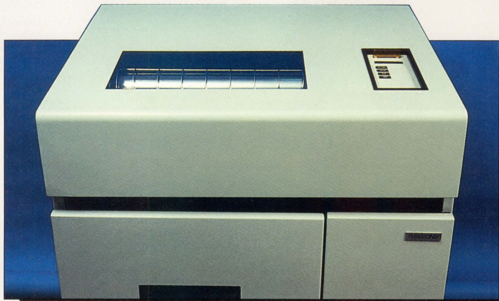
The P9012 features a straight-through, enclosed paper path for easy loading.
