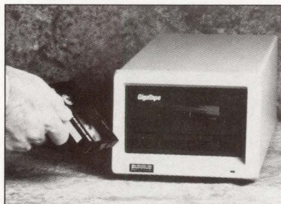
The GigaTape, in 5/4" form factor, integrates easily into high-capacity data storage systems such as our GigaBox, and uses standard 8mm data cartridges.
