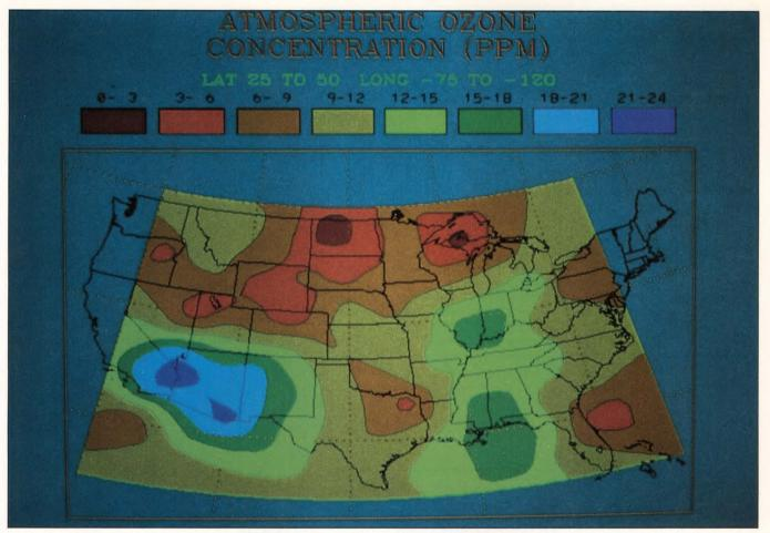
This two-dimensional map was produced by ICEX Inc., of Louisville, Colorado, using its GRAPHKit utilities, which, in turn, call GKS for graphic output. The GKS package stored the picture in a CGM file which later was displayed to produce the slide.
