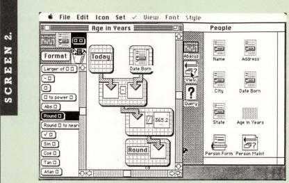
Helix computed fields are defined by selecting and arranging function "tiles." Shown is the computation of age in years, determined by subtracting date of birth from current date, dividing by 365.25 and rounding the result.
