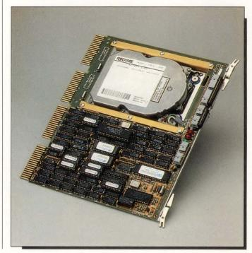
The CMD hard card. The drive projects three slots on the other side of the card. A second drive can connect to the edge connectors, but must get power elsewhere.
