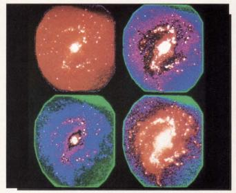
Gray scale transformation. Clockwise from top left: original image of galaxy; histogram equalized; elements less than 50 percent of transformed image's maximum; logarithmically transformed image.
