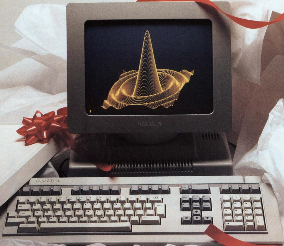
Upgrade your DEC environment with the Ditto 221XL video display terminal from Networx Data Products Co. It has all the features of the DEC VT220 plus over 11 major improvements, including superior resolution, dual host port ability and a larger screen. And with the 221GXL upgrade you can create incredible graphs, charts, plots, drawings and many other monochrome graphics . . . without disturbing any of the 221XL's alpha-numeric features.
