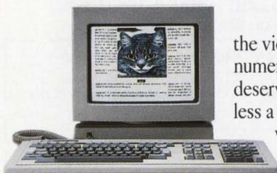
*Though it's priced like an alphanumeric terminal, our 600 Series can display both bit-mapped graphics and full-featured text.*
