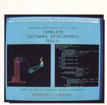
Photo 2: This promotional slide for CADIF's technology transfer workshops shows a robot modeled in HOOPS and a portion of the C code that generated it.
