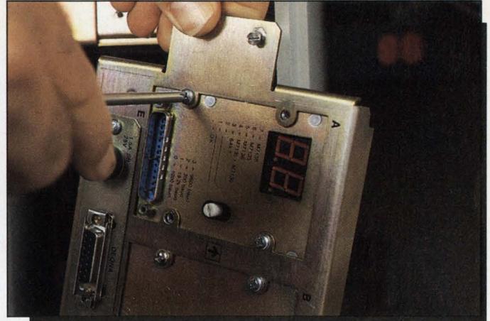
*Photo 3. Remove the old rear panel switch plate.*
