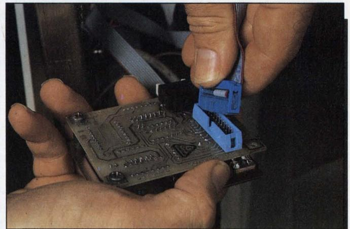
*Photo 7. Notice that the larger cable to the rear is keyed with a notch in the receptacle that mates with the cable.*
