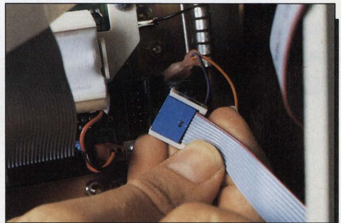
*Photo 5. The small cable between the MICROVAX II CPU and the rear panel is keyed . . .*
