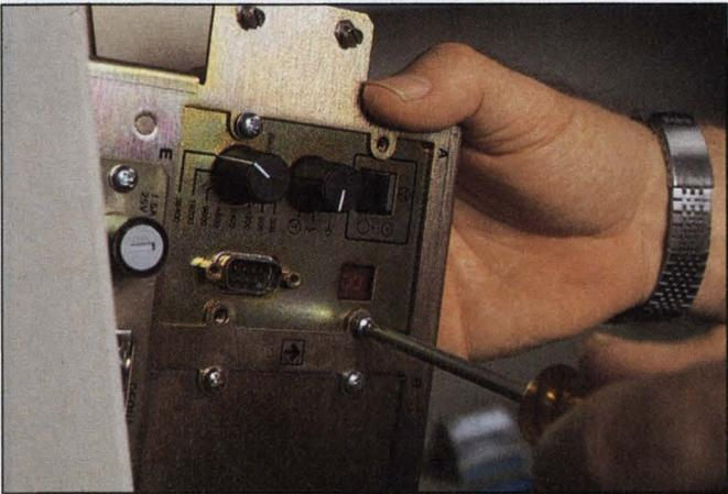
*Photo 4. Install the replacement rear panel.*
