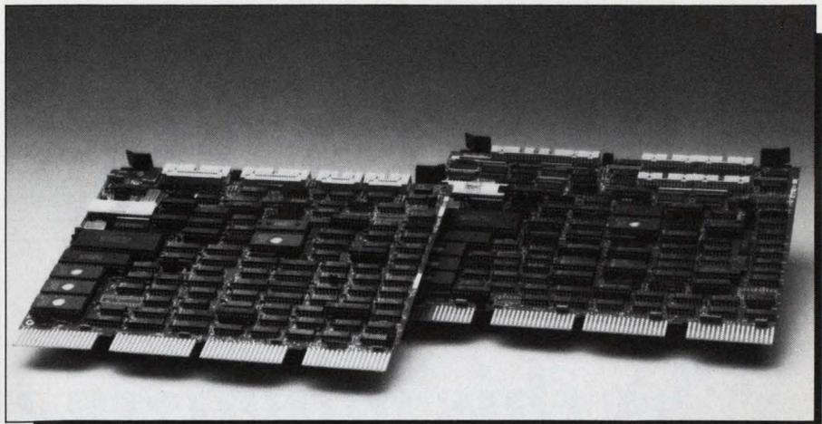
*The DCV50 and DCV54 are Plessey Peripheral Systems' new disk controllers.*
