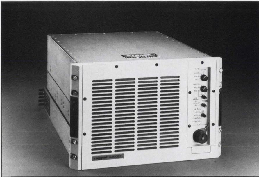
*RUGGED DIGITAL'S R/8200 ruggedized DEC VAX 8200 computer system is for military applications.*
