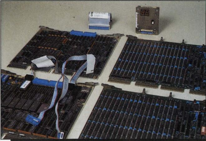
*Photo 2. Go into the BA23 and remove both MICROVAX I CPU boards, and whatever memory boards happen to be there (in this case, two). You can give these to your cousin with the PDP-11.*
