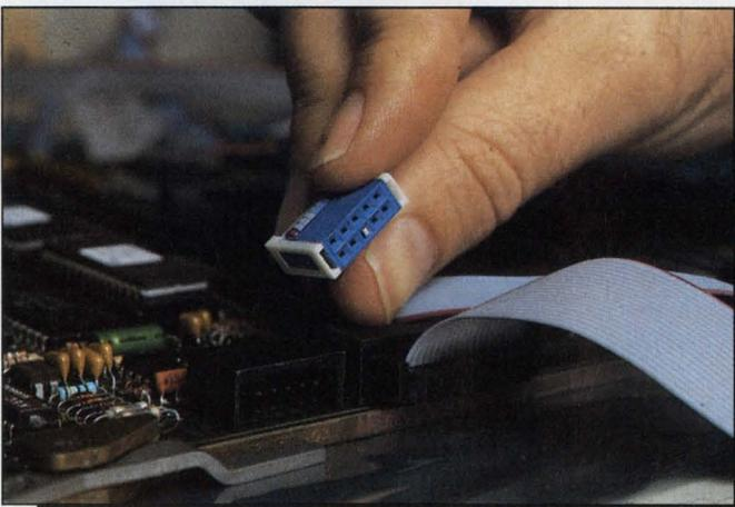
*Photo 6. . . note that the hole for the missing pin is plugged on the cable.*
