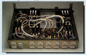
The unit has five other connectors that are the remote control inputs. If you connect pin one to pin three the unit will power up, provided the unit is set for "remote." If you short pin two to three, all three of the switched circuits, as well as the J8 remote, will disengage. This is good for power-down sensor circuits such as temperature and water. See *DEC PROFESSIONAL*, August, 1986, Vol. 5., No. 8, for a review of SAM (Smart Ambient Monitor).
