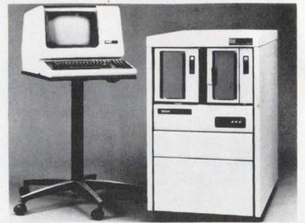
160MB fixed Winchester disk, and a companion 80MB removable cartridge disk. Choice of operating systems includes RT-11, RSX11-M or UNIX.
