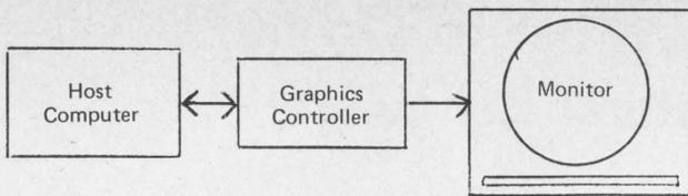
Figure 1-6: Programmable interface between host computer and monitor.
