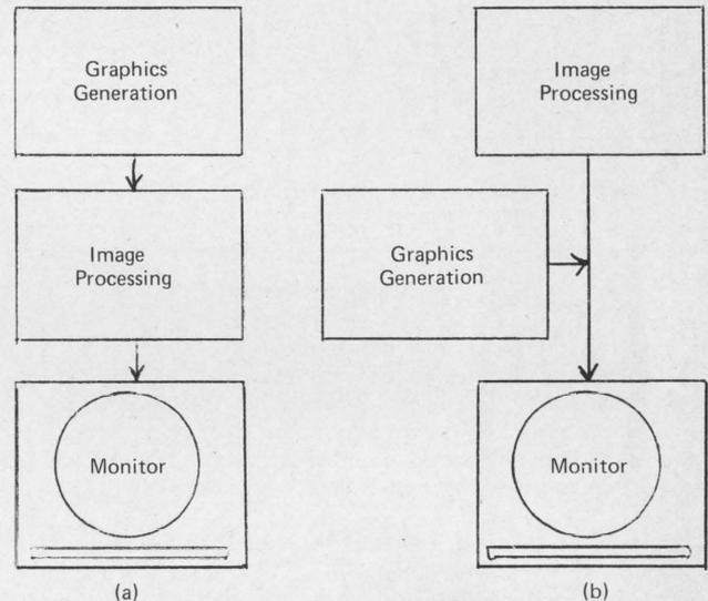
Figure 1-1: Multiple graphics and imaging functions -- performed sequentially (a) or combined on monitor screen (b).
