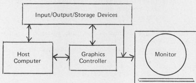
Figure 1-8: Graphics-system I/O and data-storage resources.
