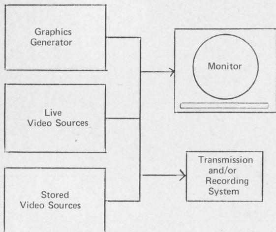
Figure 1-2: Television switching/mixing system with multiple display-signal sources.
