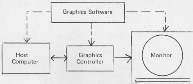
Figure 1-7: Distribution of graphics-system software functions.
