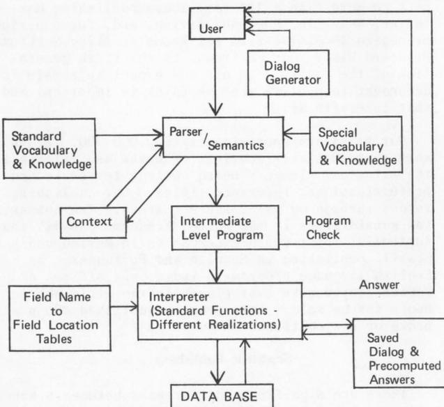
Figure 4: Block Diagram of PLANES
