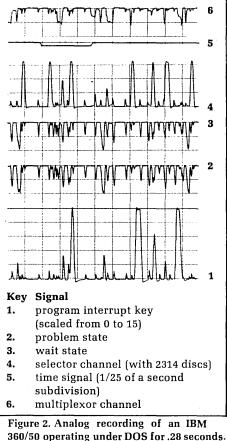
• ANALOG. Like a stethoscope, analog devices are attached at various points in a computer system and signals, generally voltage readings, are recorded continuously on some type of recording surface, usually a strip chart, as illustrated in Figure 2. Voltage changes in CPU circuits or data channels indicate the activity level of the system at
